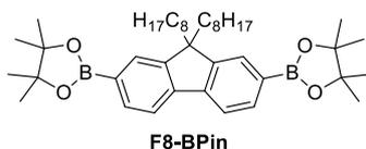
Prepared from **4a** (10.00 g, 18.23 mmol) according to the general procedure. The crude product was purified by column chromatography (stationary phase: silica, eluent: hexane/methylene chloride 4:1) and the product **F8-BPin** (8.00 g, 12.45 mmol, 68 %) was obtained as a white solid. <sup>1</sup>H-NMR (400 MHz, CDCl<sub>3</sub>) δ [ppm] = 7.83 (dd, *J* = 7.5 Hz, 0.9 Hz, 2H), 7.79 – 7.72 (m, 4H), 2.06 – 1.98 (m, 4H), 1.41 (s, 24H), 1.25 – 0.98 (m, 20H), 0.83
