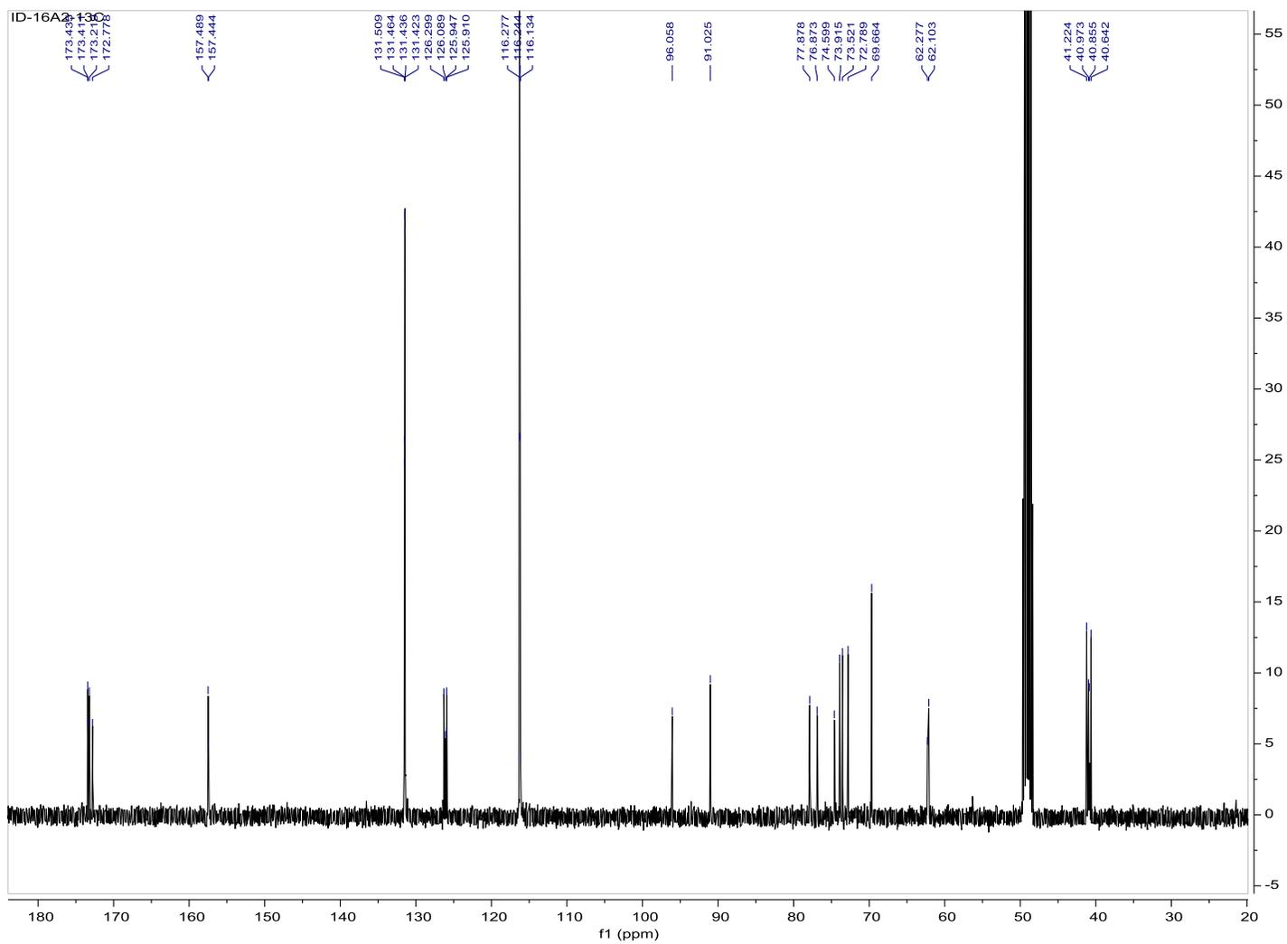
Figure S12  $^{13}\text{C}$ -NMR spectrum of compound 2 (methanol- $d_4$ )
