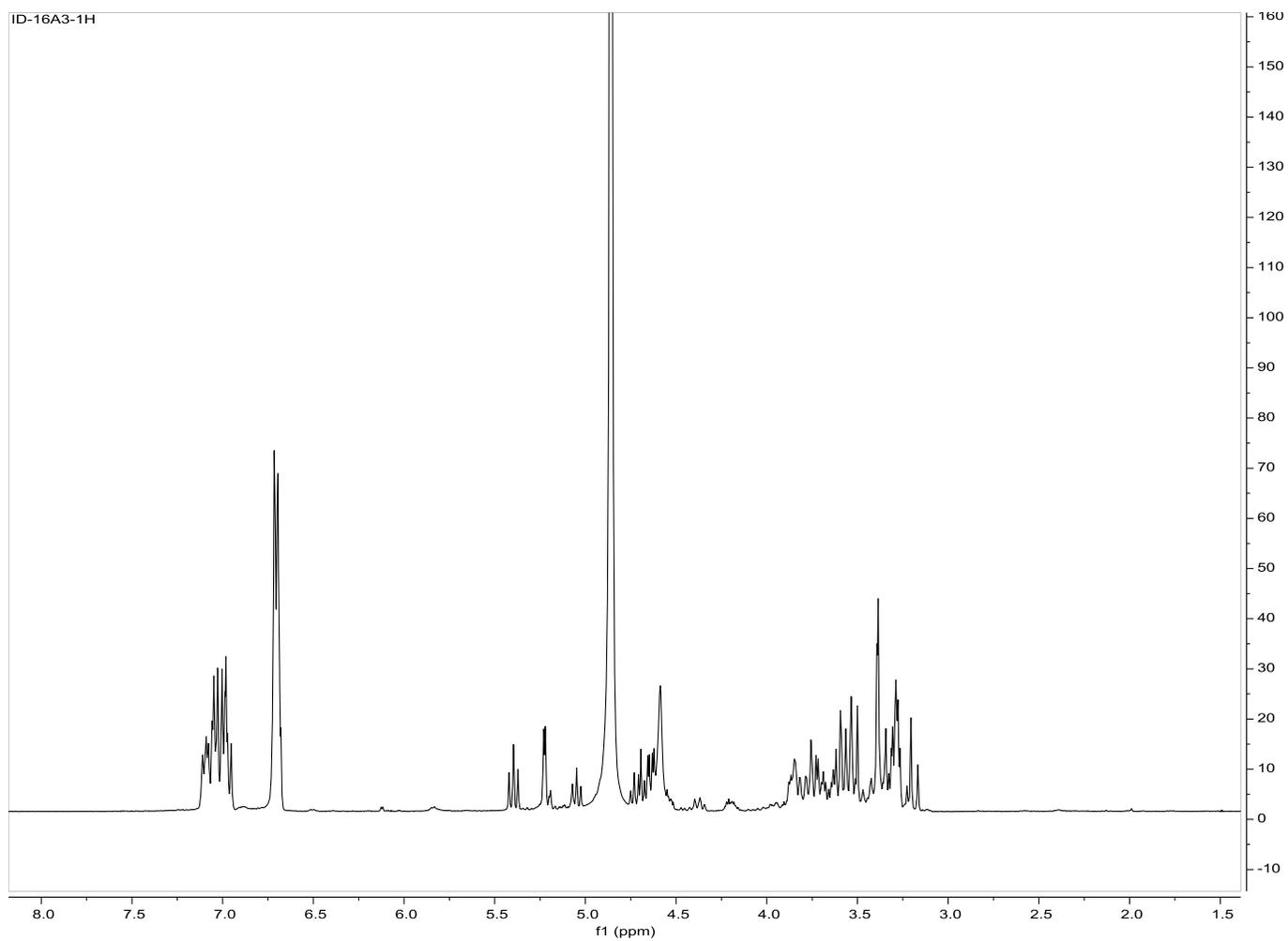
**Figure S11**  $^1\text{H-NMR}$  spectrum of compound **2** ( $\text{methanol-}d_4$ )
