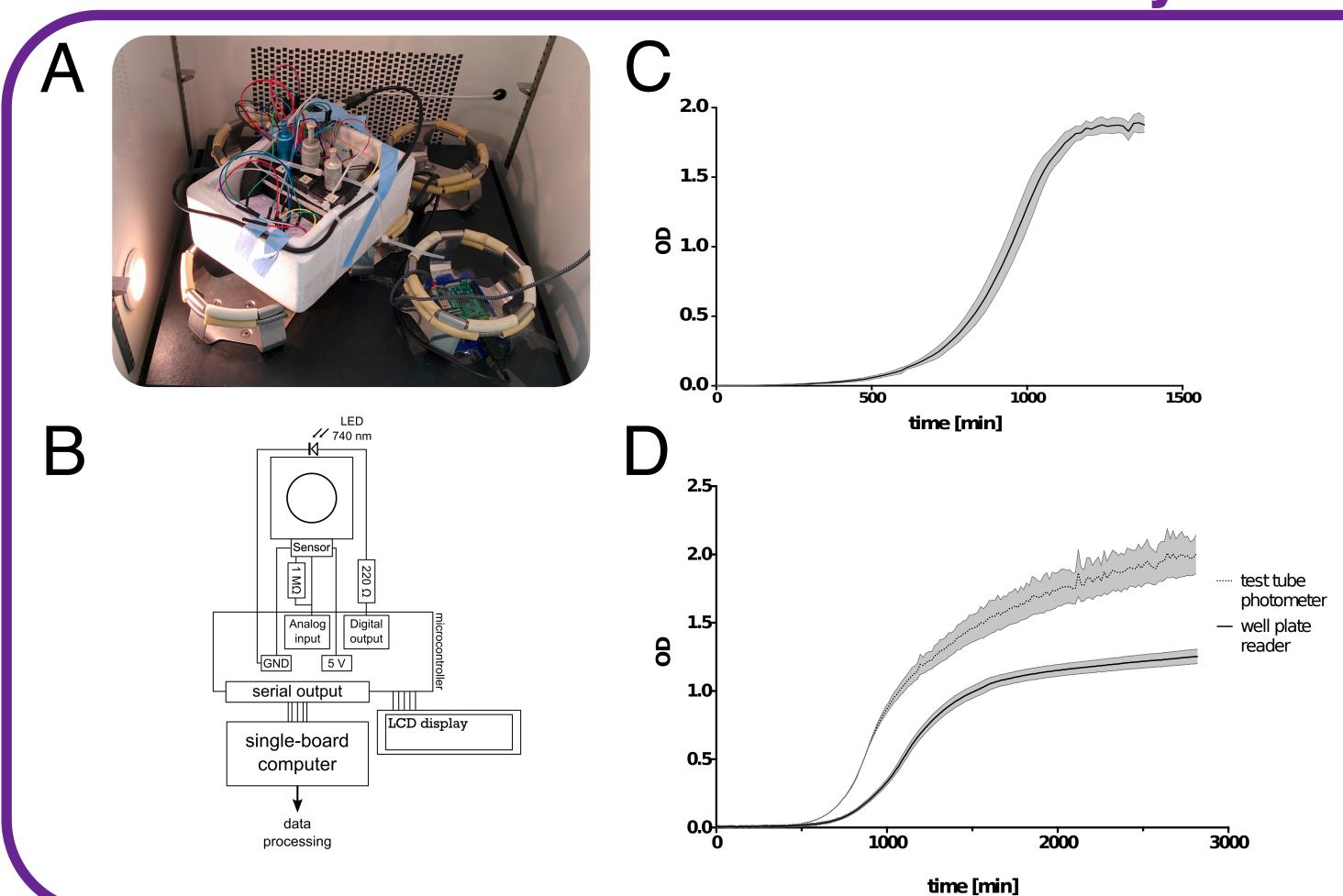
How about skipping the sample taking and transferring step and measure the culture density directly in the test tube? We developed a test tube photometer based on an LED, a highly sensitive photodiode and a microcontroller (**A**, **B**). The 3D-printed housing can be adjusted to fit any test tube size.
