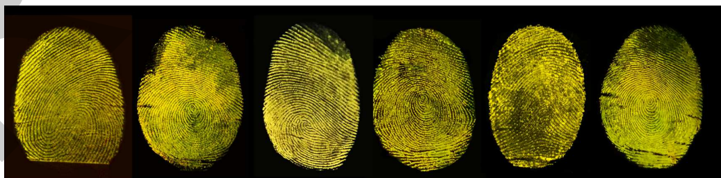
Figure S9 The fluorescent images of LFPs deposited on glass slides by different people under an UV lamp (where \lambda_{ex}=365 nm).
