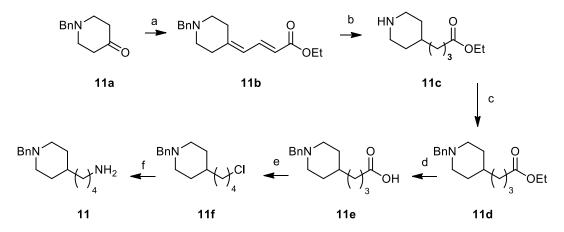
Scheme for 11 synthesis. *Reagents and conditions*<sup>1</sup>: (a) (EtO)<sub>2</sub>P(O)CH<sub>2</sub>CH=CHCO<sub>2</sub>Et, EtOH, NaH, Reflux, 1h; (b) H<sub>2</sub>, Pd/C 10%, 40mbarr, EtOH, RT O.N.; (c) BnBr, Et<sub>3</sub>N, CH<sub>2</sub>Cl<sub>2</sub>, O.N.; (d) LiAlH<sub>4</sub>, dry THF, reflux, 2h; (e) SOCl<sub>2</sub>, CH<sub>2</sub>Cl<sub>2</sub>, reflux, 3h; (f) NH<sub>3</sub>/MeOH 7M, 5mbarr, 5h.
