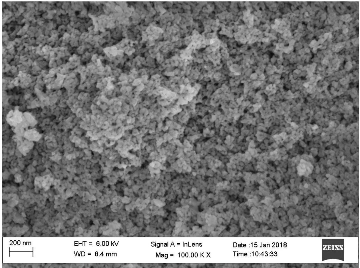
**Figure S1.** FE-SEM image of a nanostructured screen-printed bare NiO sample
