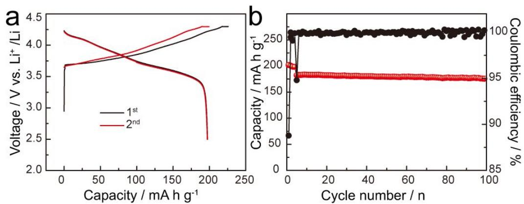
**Figure S6.** (a) charge and discharge curves of  $\text{LiNi}_{0.8}\text{Co}_{0.1}\text{Mn}_{0.1}\text{O}_2$  in half cell, (b) cycling stability and CE of  $\text{LiNi}_{0.8}\text{Co}_{0.1}\text{Mn}_{0.1}\text{O}_2$  in half cell.
