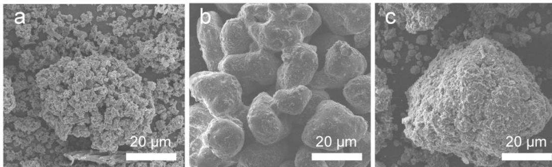
**Figure S2.** (a) SEM image of composites after reacting at 350 °C under 2 MPa, (b) SEM image of composites after reacting at 480 °C under 4 MPa, (c) SEM image of composites after reacting at 430 °C under 2 MPa.
