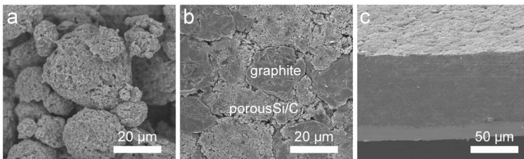
**Figure S5.** SEM image of (a) Si/C microspheres with porous structure fabricated by spray-drying, (b) top view of electrode prepared with Si/C microspheres and graphite, (c) cross-section view of electrode prepared with Si/C microspheres and graphite.
