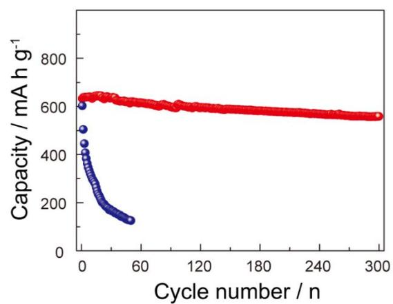
**Figure S3.** Cycling performance of Si/C microspheres (red) and mixture (blue) at 0.2 C.
