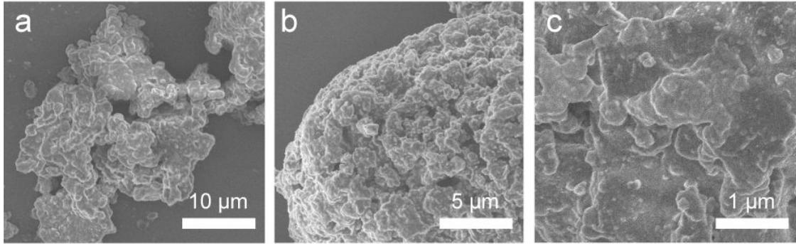
**Figure S1.** (a) Typical SEM image of Si NPs anchored on the graphite with pitch, (b) high-resolution (HR-) SEM image of composites after 1.5 h reaction, (c) HR-SEM image of surface of Si/C microsphere.
