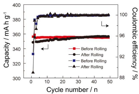
**Figure S4.** Electrochemical performance of commercial graphite before and after rolling process.
