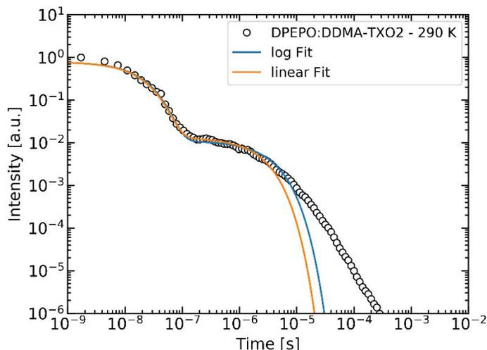
**Figure S3:** Comparison of log fit (restricted dataset, default starting parameters) and linear fit (unrestricted dataset, starting parameters preceding log fit).
