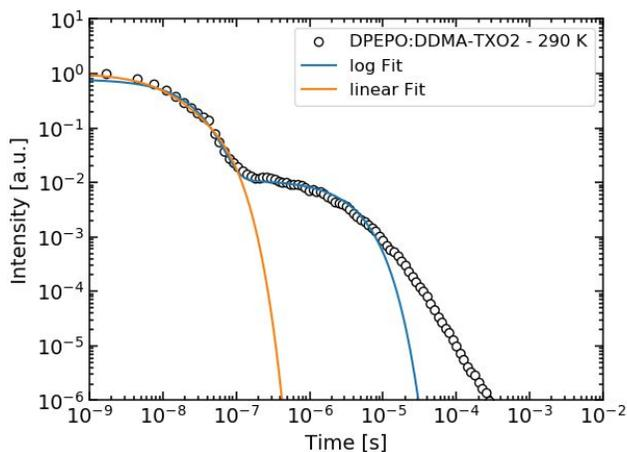
**Figure S1:** Comparison of linear (unrestricted dataset) and log (restricted dataset) fits to decay data, using same initial parameter values.
