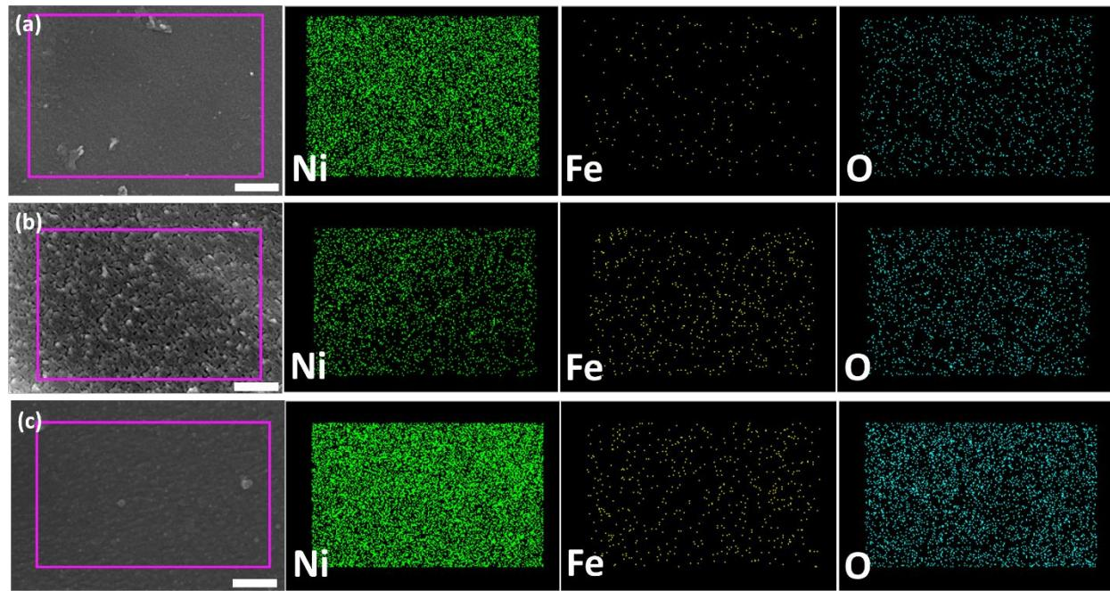
Fig. S9 Elemental mapping of samples: (a) 0.08M Fe/A-NF, (b) 0.14M Fe/A-NF, (c) 0.2M Fe/A-NF.
