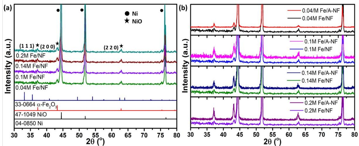
Fig. S2 (a) XRD patterns of annealed samples after anodization without  $\text{NH}_4\text{F}$ . (b) Comparison of annealed samples after anodization with (/A-NF series) and without (/NF series)  $\text{NH}_4\text{F}$ .
