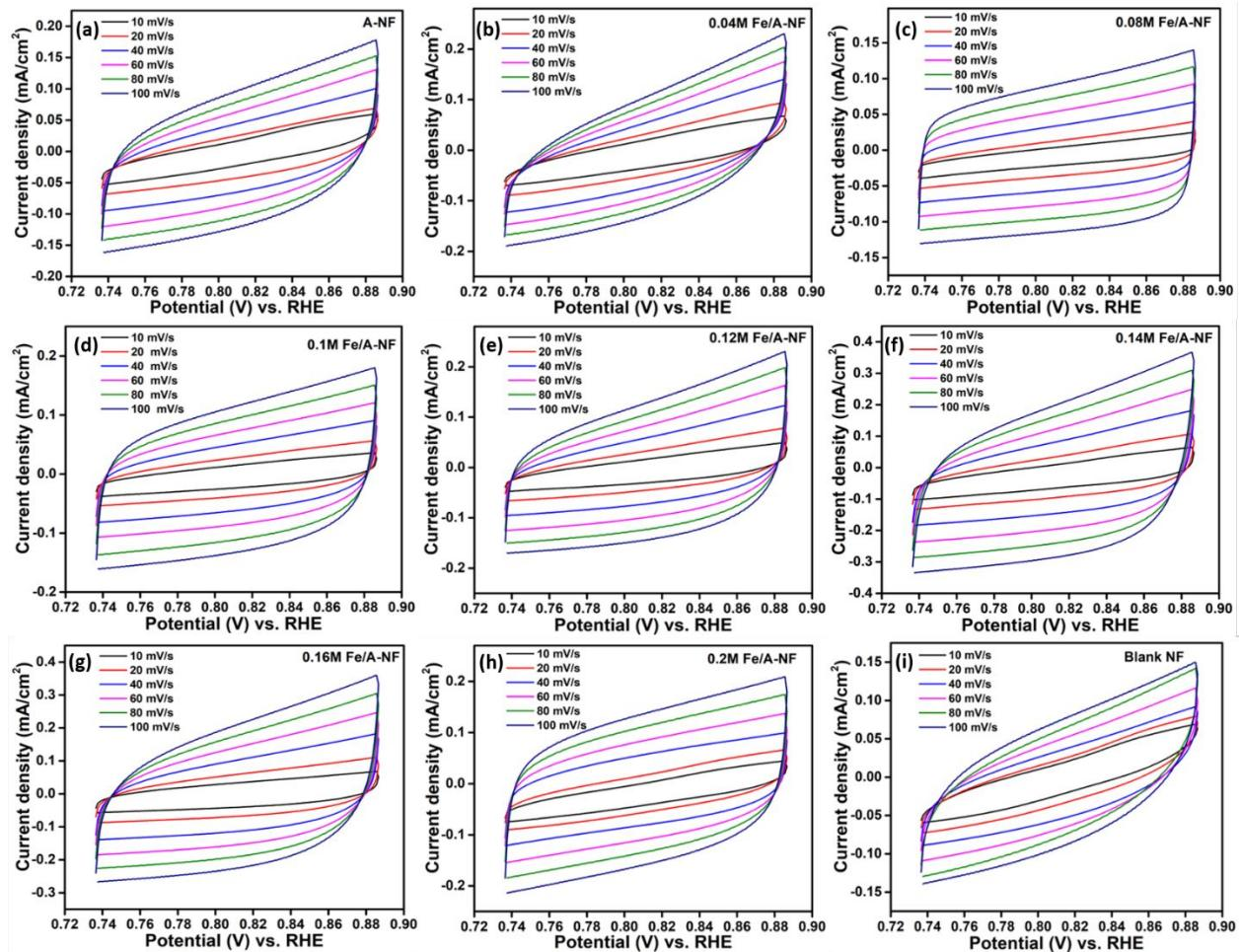
Fig. S12 Cyclic voltammograms recorded at increasing scan rates in 1M KOH of (a) A-NF, (b) 0.04M Fe/A-NF, (c) 0.08M Fe/A-NF, (d) 0.1M Fe/A-NF, (e) 0.12M Fe/A-NF, (f) 0.14M Fe/A-NF, (g) 0.16M Fe/A-NF, (h) 0.2M Fe/A-NF, (i) blank NF.
