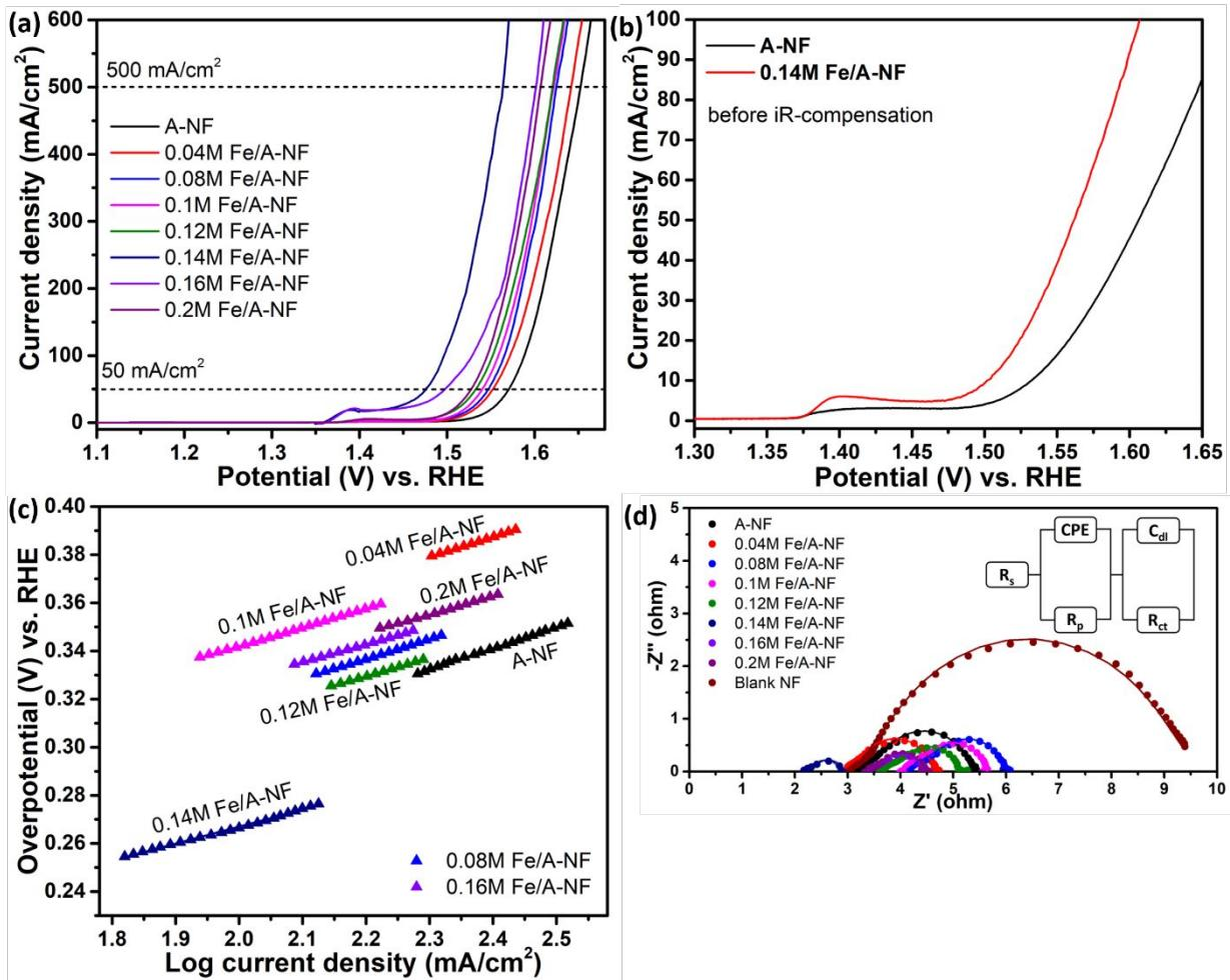
Fig. S10 OER activities of electrodes. (a) LSV polarization curves. (b) LSV polarization curves without iR-compensation. (c) Tafel slopes. (d) Nyquist plots recorded at 1.64 V vs. RHE, inset: equivalent circuit model.
