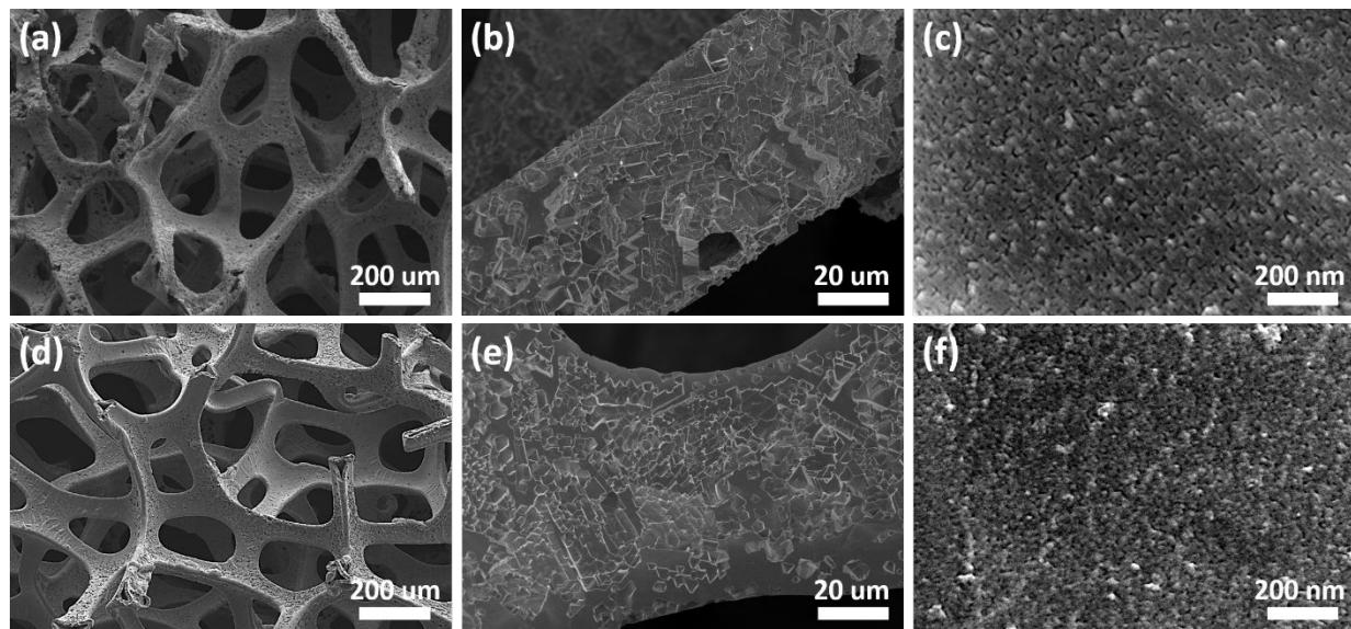
Fig. S15 SEM images of (a), (b), (c) sample 0.14M Fe/A-NF before chronoamperometric stability test, and (d), (e), (f) after chronoamperometric stability test at 500 mA/cm<sup>2</sup> for 24 hrs as anode.
