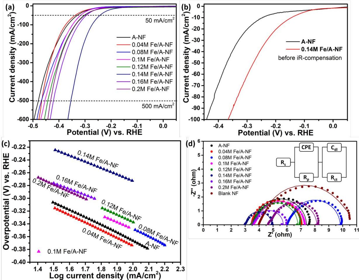
Fig. S11 HER activities of electrodes. (a) LSV polarization curves. (b) LSV polarization curves without iR-compensation. (c) Tafel slopes. (d) Nyquist plots recorded at -0.31 V vs. RHE, inset: equivalent circuit model.
