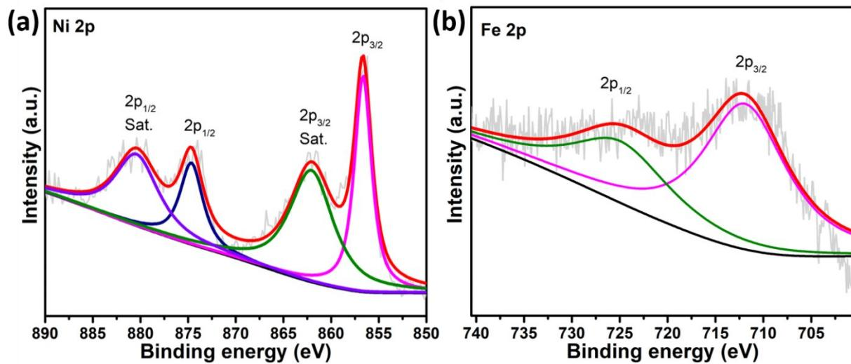
Fig. S17 HRXPS spectrum of sample 0.14M Fe/A-NF after chronoamperometric stability test at 500 mA/cm<sup>2</sup> for 24 hrs as cathode: (a) Ni 2p and (b) Fe 2p.
