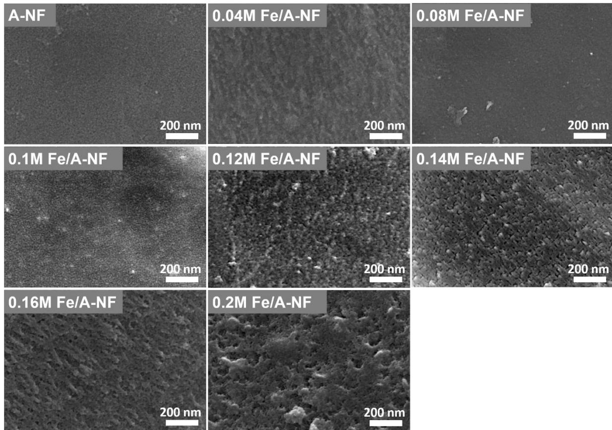
Fig. S5 SEM images of anodized samples at magnification of 100k.
