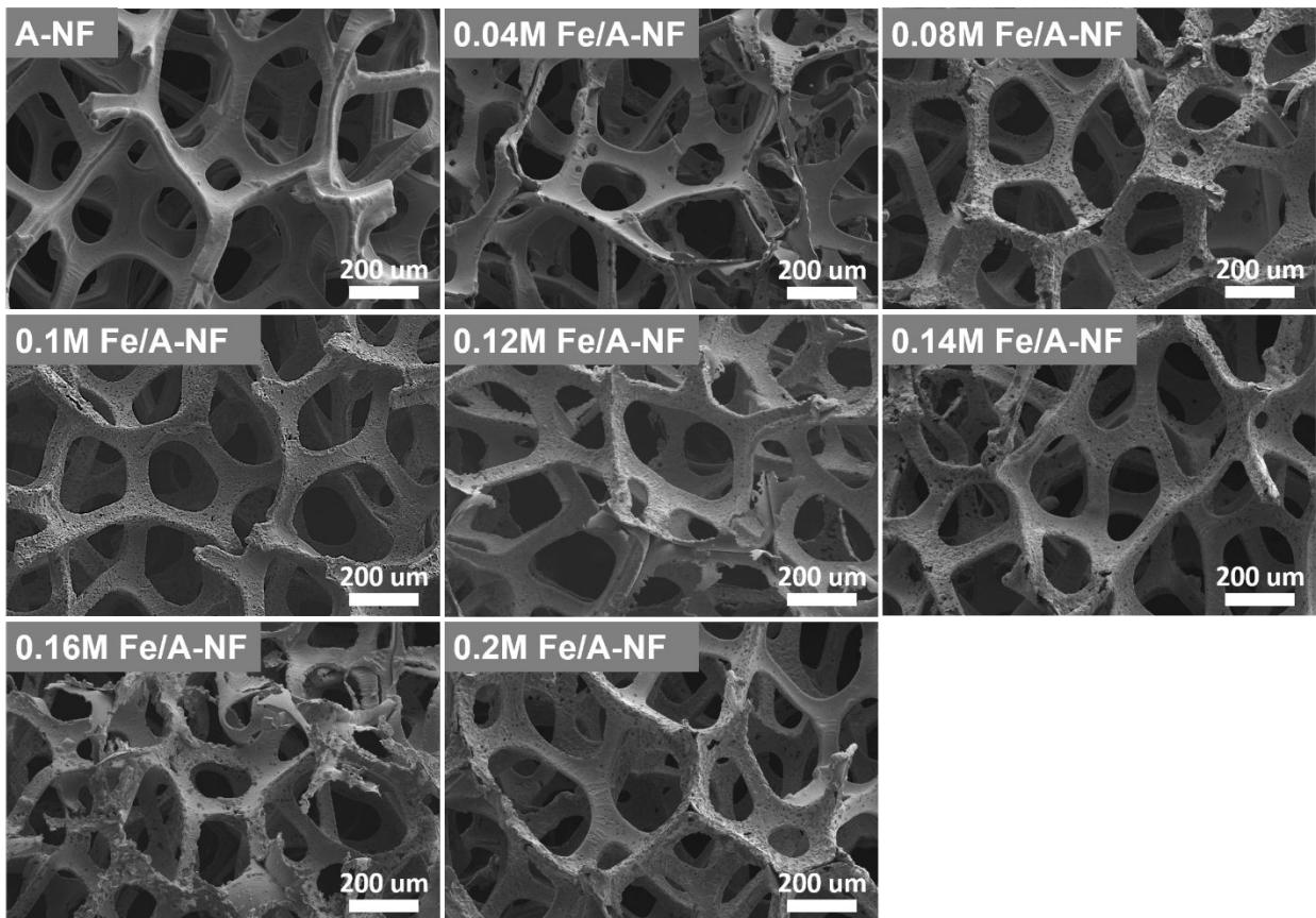
Fig. S3 SEM images of anodized samples at magnification of 100.
