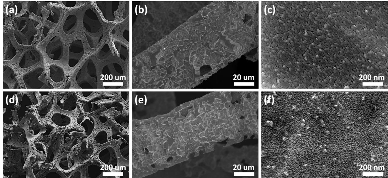
Fig. S14 SEM images of (a), (b), (c) sample 0.14M Fe/A-NF before chronoamperometric stability test, and (d), (e), (f) after chronoamperometric stability test at  $500 \text{ mA}/\text{cm}^2$  for 24 hrs as cathode.
