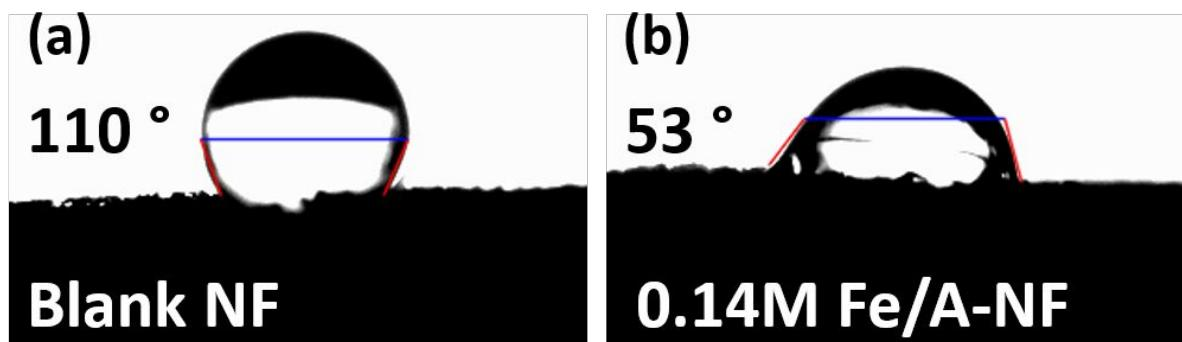
Fig. S20 Static contact angle measurements for (a) blank NF and (b) sample 0.14M Fe/A-NF, showing hydrophilic nature of both samples.
