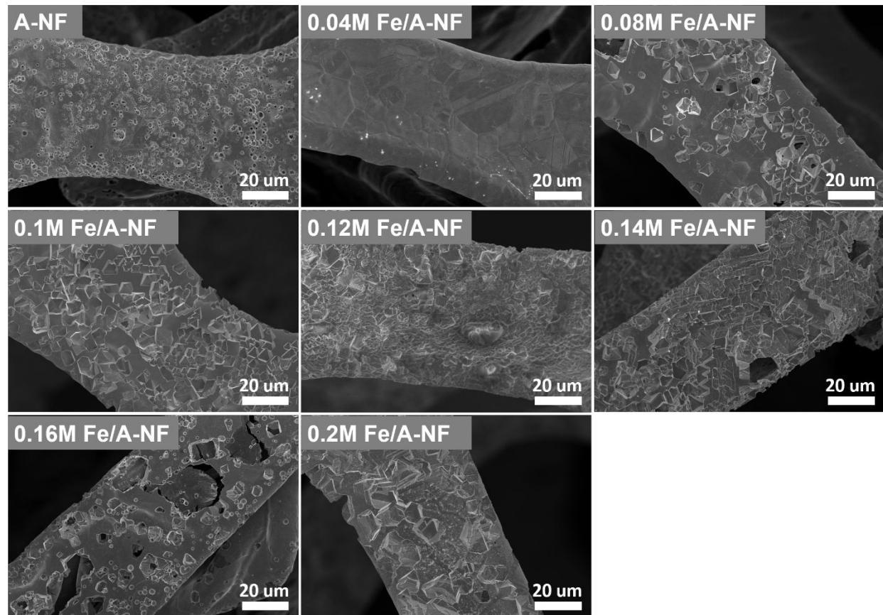
Fig. S4 SEM images of anodized samples at magnification of 1k.
