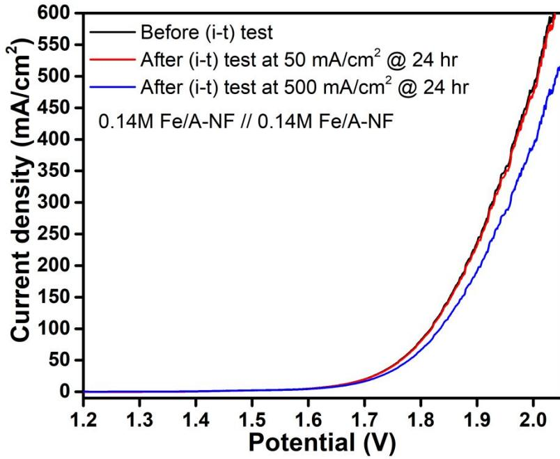
Fig. S13 LSV polarization curves of 0.14M Fe/A-NF//0.14M Fe/A-NF couple before and after chronoamperometric stability test for 24 hrs.
