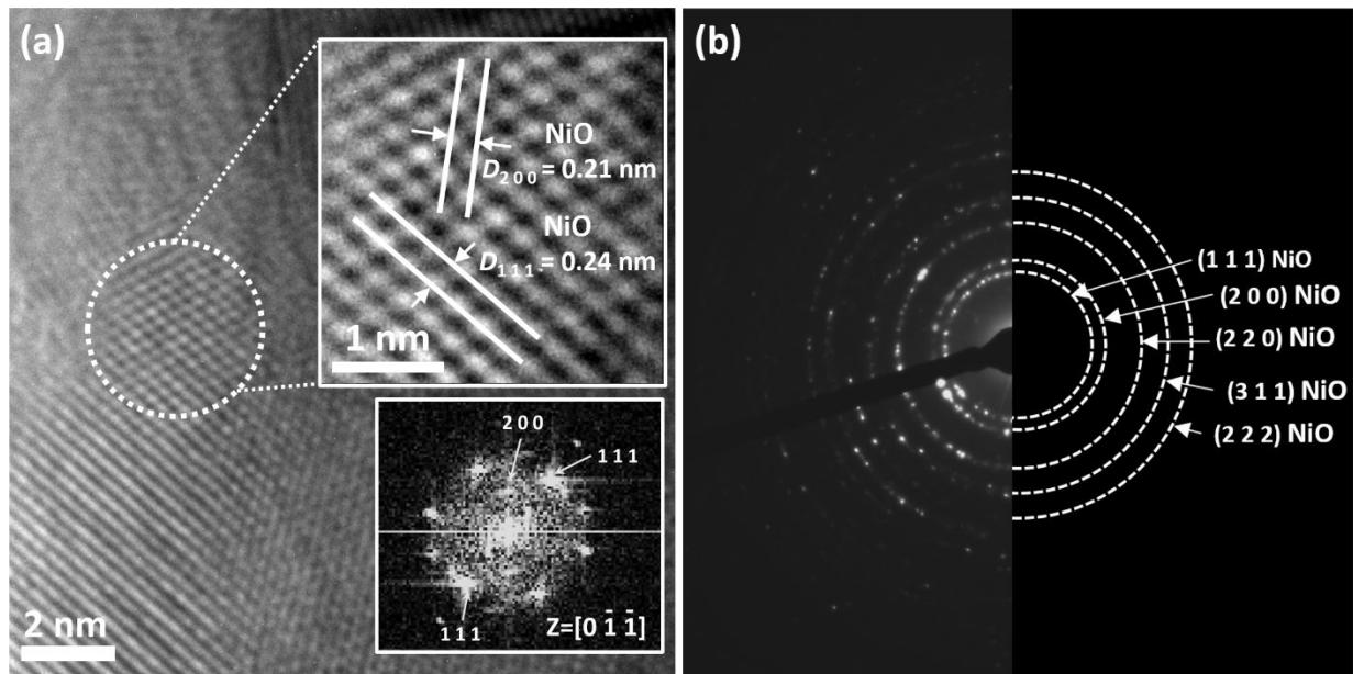
Fig. S7 (a) HRTEM image of A-NF, insets: locally enlarged HRTEM of white circled region and corresponding FFT pattern obtained from white circled region. (b) SAED patterns of A-NF.
