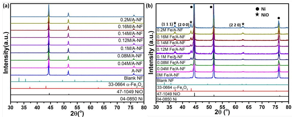
Fig. S1 (a) XRD patterns of anodized electrodes. (b) XRD patterns of anodized electrodes annealed under Argon atmosphere to confirm formation of oxide layer.
