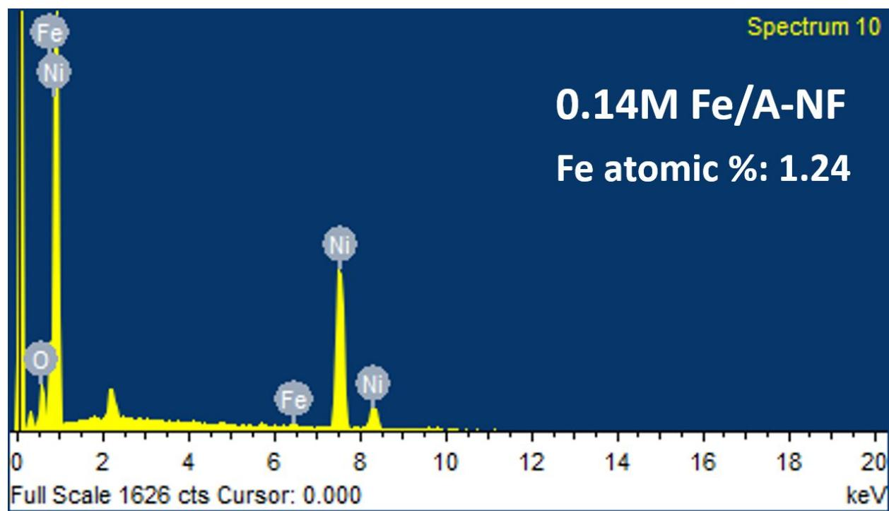
Fig. S8 EDX spectrum of sample 0.14M Fe/A-NF, confirming presence of Fe in sample.
