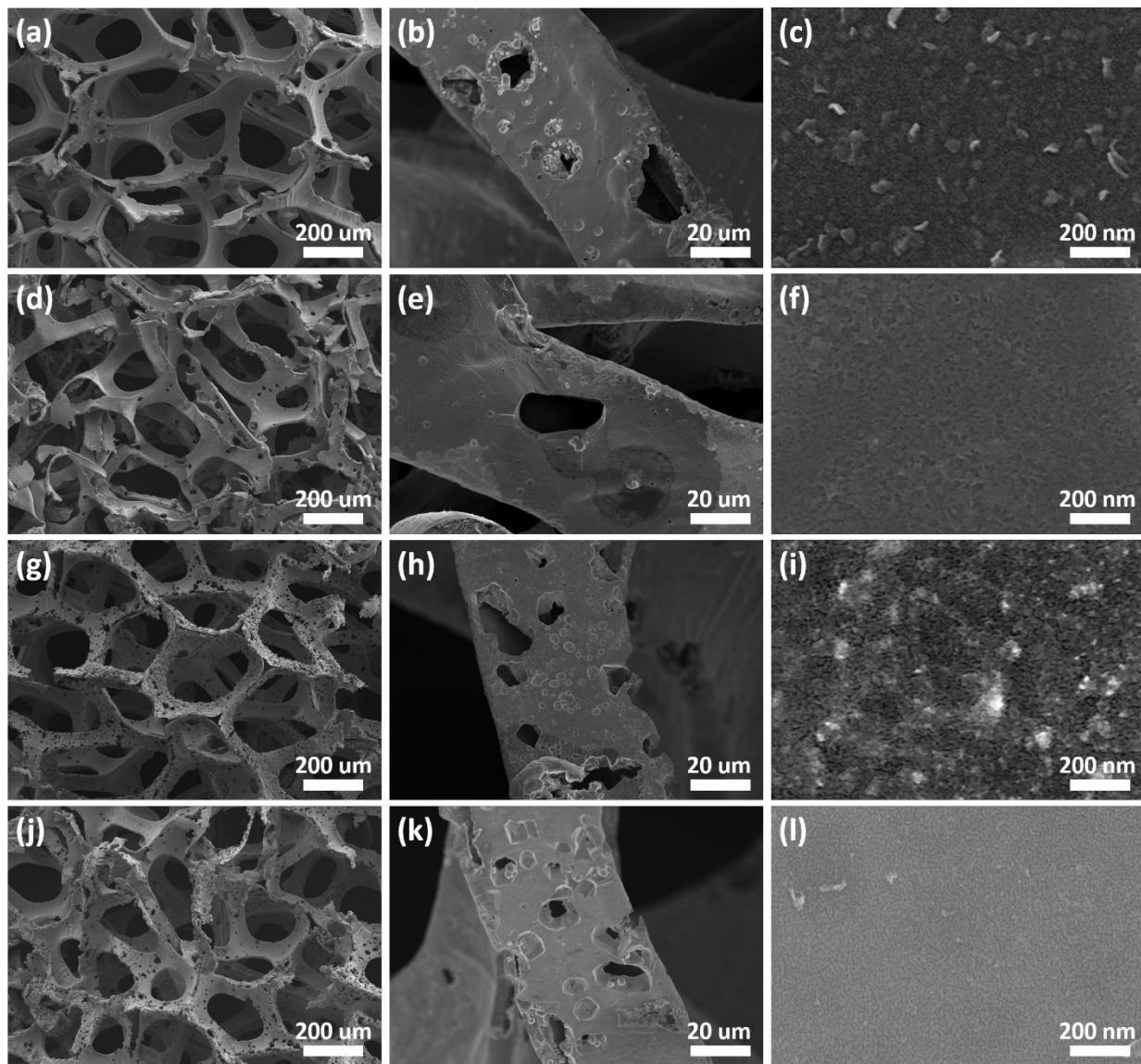
Fig. S6 SEM images of (a), (b), (c) 0.04M Fe/NF, (d), (e), (f) 0.1M Fe/NF, (g), (h), (i) 0.14M Fe/NF, and (j), (k), (l) 0.2M Fe/NF.
