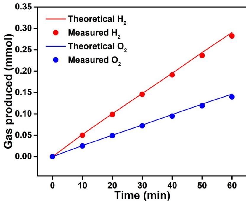
Fig. S19 Experimental and theoretical amounts of H<sub>2</sub> and O<sub>2</sub> production by 0.14M Fe/A-NF//0.14M Fe/A-NF couple for overall water splitting at 80 mA/cm<sup>2</sup>.
