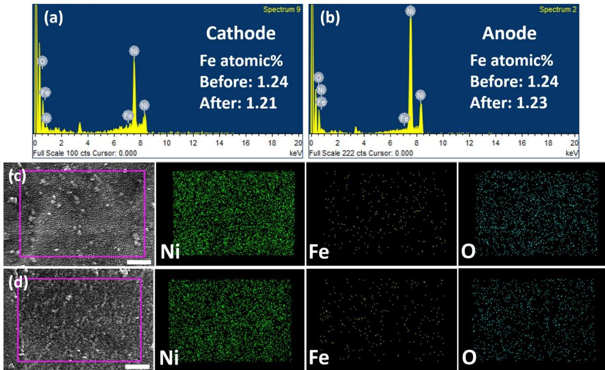
Fig. S16 EDX spectra of sample 0.14M Fe/A-NF after chronoamperometric stability test at 500 mA/cm<sup>2</sup> for 24 hrs: (a) as cathode and (b) as anode. Elemental mapping of sample 0.14M Fe/A-
