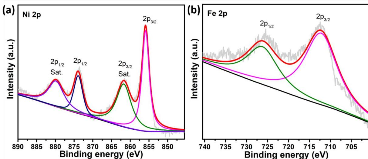
Fig. S18 HRXPS spectrum of sample 0.14M Fe/A-NF after chronoamperometric stability test at 500 mA/cm<sup>2</sup> for 24 hrs as anode: (a) Ni 2p and (b) Fe 2p.
