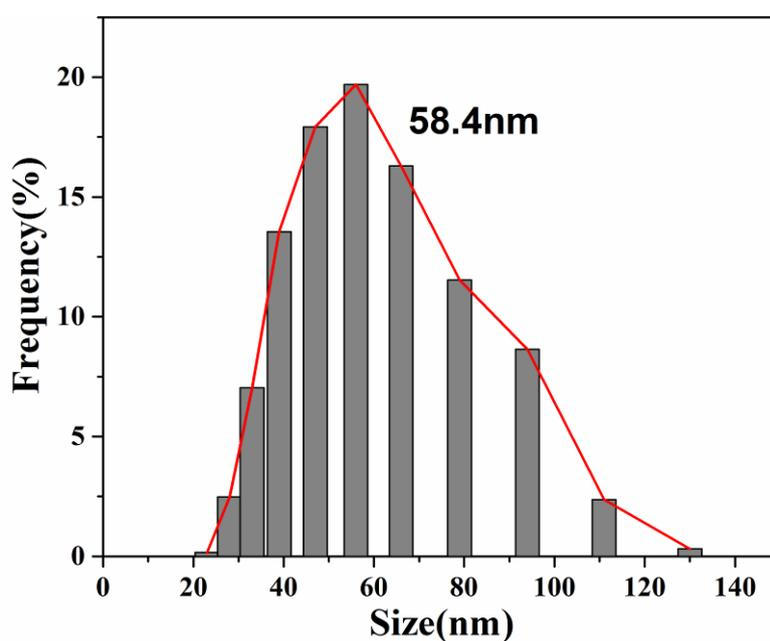
**Figure S4.** The hydrated particle size distribution of PEG- $\text{CeO}_2:\text{Gd}$  in water by dynamic light scattering (DLS) measurement. DLS showed that the hydrated size of PEG- $\text{CeO}_2:\text{Gd}$  is 58.4 nm (PDI = 0.165), and the zeta potential is +19.8 mV.
