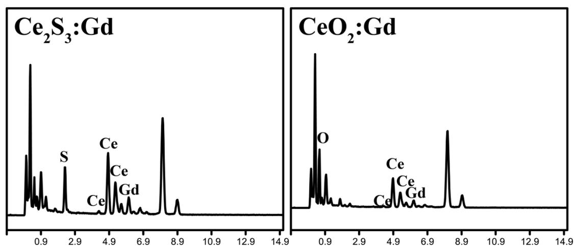
**Figure S1.** The elemental analysis of  $\text{Ce}_2\text{S}_3:\text{Gd}$  and oxidated PEG- $\text{CeO}_2:\text{Gd}$  were measured by TEM-EDS.
