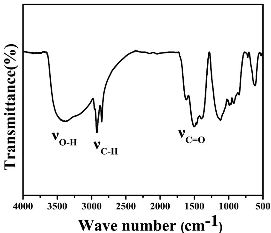
**Figure S2.** The FT-IR spectrum of PEG-modified PEG- $\text{CeO}_2:\text{Gd}$ . The broad band at about  $3450 \text{ cm}^{-1}$  is attributed to the O–H stretching vibration of adsorbed water and/or
