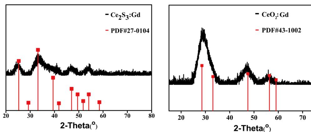
**Figure S3.** The XRD pattern shows that the as-synthesized Gd ions doping  $\text{Ce}_2\text{S}_3$  (JCPDS No.27-0104) changed into ultra-small Gd ions doping  $\text{CeO}_2$  (JCPDS No.43-1002) after hydrolysis reaction.
