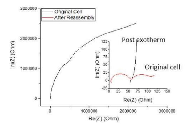
Figure S11: Impedance measurement of NCA after the exothermic reaction at 4.75V and 60  $^{\circ}$ C. A very large rise in impedance rise has been observed at this condition which is due to transition metal cation (Ni<sup>+2</sup>, Co<sup>+2</sup>) dissolution and plating on to the anode. The impedance drops sharply after the anode is substituted with a new one indicating that the large impedance rise can be attributed to the anode.
