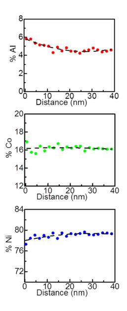
Figure S10: X-Ray EDS concentration profile of pristine NCA showing concentration profile (at.%) of (a) Al, (b) Ni and (c) Co revealing an Al enrichment at the surface from 4.5 to 6%.
