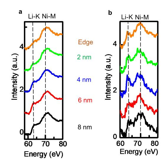
Figure S5: The low loss spectra as a function of distance in the area with (a) the layered and (b) RS contrast. The Li content is lower at the surface. In the "RS-like" area the intensity of Li(K) edge does not vary as a function of distance from the edge. In addition, the Li content appear the same or is higher than that in the layered structure.
