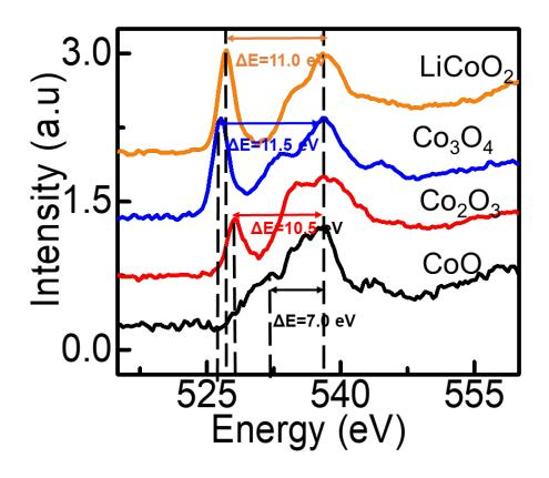
Figure S7: Characteristic EELS spectra of various cobalt oxides corresponding to layered (R $\overline{3}$ m) LiCoO<sub>2</sub>, spinel (Fd $\overline{3}$ m) Co<sub>3</sub>O<sub>4</sub>, trigonal (R $\overline{3}$ c) Co<sub>2</sub>O<sub>3</sub> and rocksalt (Fm $\overline{3}$ m) CoO. Spinel and layered structures have similar EELS characteristics.
