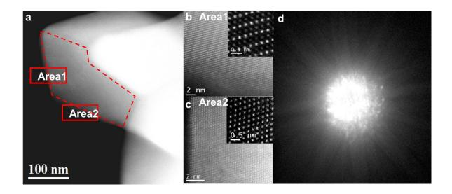
Figure S2: Presence of layered and rocksalt-type contrasts in a single particle. (a) The dashed region comprises two facets marked as area 1 and area 2 which shows two types of contrast. (b, c) The high magnification image of area 1 (rocksalt contrast) and area 2 (layered contrast). (d) The CBED pattern used to tilt this region along [110] layered is shown in d.
