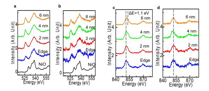
Figure S4: The core loss spectra as a function of distance in the area with (a,c) the layered and (b,d) RS contrast. Figures a, b depict O-K edge and figures c,d show the Ni-L edge. For O-K edge NiO spectrum is shown below as a reference. In case of figure c, there is shift in Ni-L edge indicating reduction at the surface.
