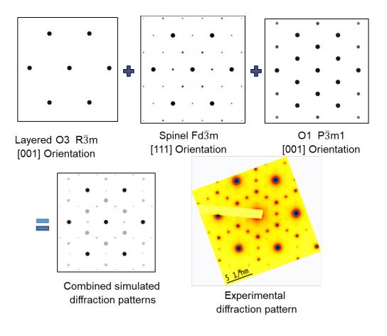
Figure S12: Simulated and experimental electron diffraction patterns of NCA held at 4.75 V and at 60 °C for 120 hours. The diffraction pattern can be indexed as the superposition of three phases with topotactic relationship corresponding to O3 ( $R\overline{3}m$ ) ZA [001], spinel ( $Fd\overline{3}m$ ) ZA [111], and O1 ( $P\overline{3}m1$ ) ZA [001]. In the experimental SAED pattern, the very weak spots close to the transmitted beam are from double diffraction.
