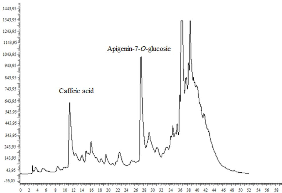
**Figure S4:** HPLC chromatogram of caffeic acid and apigenin-7-O-glucoside isolated.
