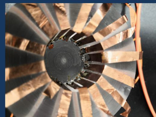
Figure 5. Inside of a prototype resistive-type sensor cell at a 5x scale. There are eight pairs of electrodes to observe the degree of radial symmetry of the reaction zone. The difficulty in fabrication means different techniques (photolithography, etching) will be required to produce the sensor at smaller scales
