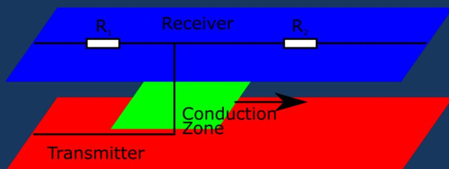
Figure 4. In resistive sensing the conduction zone acts as a potential divider of a receiver electrode. The relative sizes of the resistances behind and ahead of the detonation  $R_1$  and  $R_2$  gives the position of the rear of the conduction zone.
