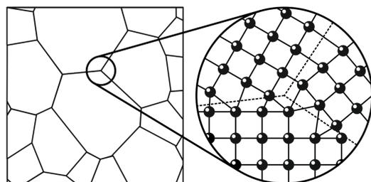
**Fig. 1:** Schematic depiction of a polycrystal. A polycrystal comprises a great number of single crystallites (or grains) within which all atoms are arranged in a regular lattice.
