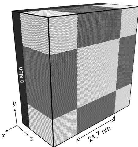
**Fig. 2:** Front end of the computational cell used in molecular dynamics simulations of a shock-compressed columnar polycrystal. The system was visualised with Ovito [1].
