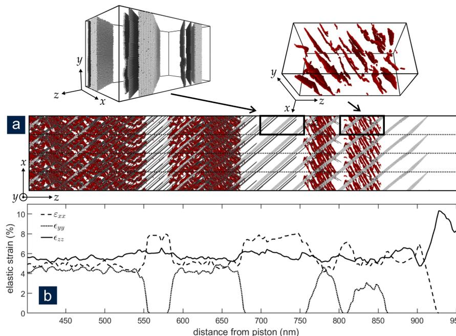
**Fig. 4:** Response of single crystal shock-loaded along the z-direction to 40 GPa. (a) Atoms located in proximity to slip or twin planes. White and grey atoms experience relative motion in the xz-plane, red in the xy-plane. (b) Elastic strains along the x-, y-, and z-directions as a function of distance along the crystal. The strain quantifies how closely spaced atomic planes are in each direction.
