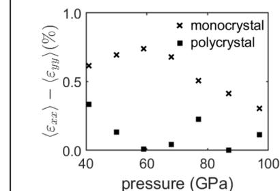
**Fig. 7:** Difference between the two transverse components of elastic strain as a function of pressure for the monocrystal and the polycrystal.
