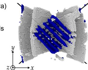
**Fig. 6:** transverse twinning in a grain in a polycrystal shocked to 60 GPa.
