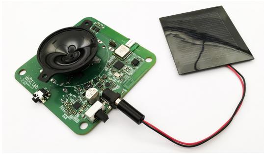
(a) Hardware PCB design with external solar panel.
