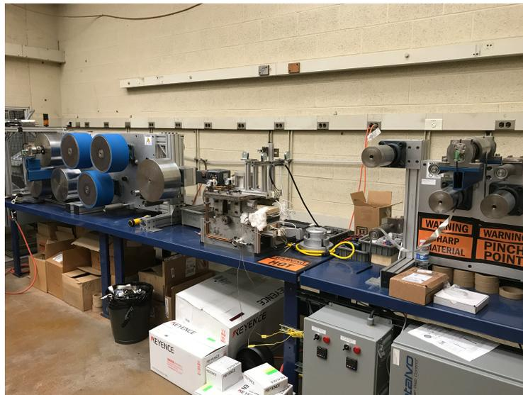
Figure 3.10: The large-scale strain-annealer at CMU. The furnace can be seen in the center, and tension rollers are located on the sides.
