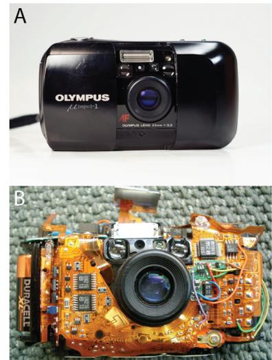
Figure 1.3: Olympus MJU I Infinity Stylus  $\mu$  (A) Popular circa 1991 fully automatic compact camera made by Olympus. (B) Rigid exterior (hard case) is removed to expose the flexible circuit assembly that is wrapped around the camera body.
