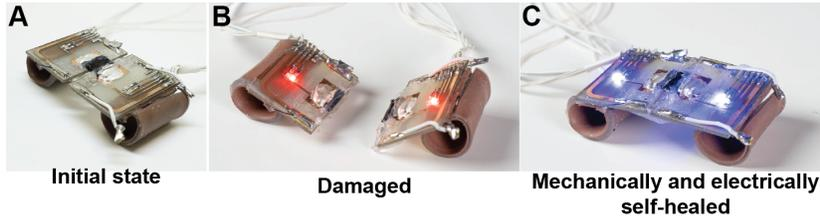
Figure 6.7: Example of a next generation soft robot that is capable of both mechanically and electrically self-healing. (A) Original state of the soft robot. (B) The soft robot is cut in half using a razor blade. (C) The two halves of the soft robot are manually rejoined to facilitate both mechanical and electrical self-healing.
