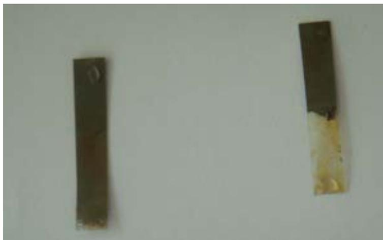
Figure 2.7 Degradation of nickel coating on PET substrate after 16 days immersion in an isopropanol based electrolyte solution. The two samples are duplicates of each other.
