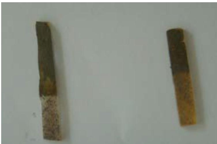
Figure 2.6 Degradation of nickel coating on glass substrate after 16 days immersion in an isopropanol based electrolyte solution. The two samples are duplicates of each other.
