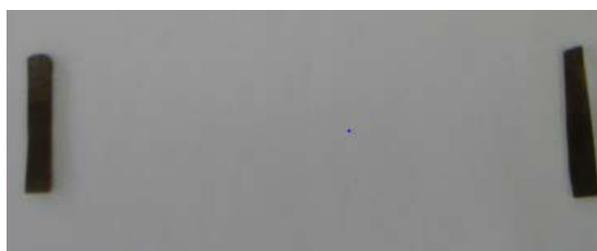
Figure 2.8 Nickel coating on glass substrate intact after 109 days immersion in an ionic liquid based electrolyte solution. The two samples are duplicates of each other.
