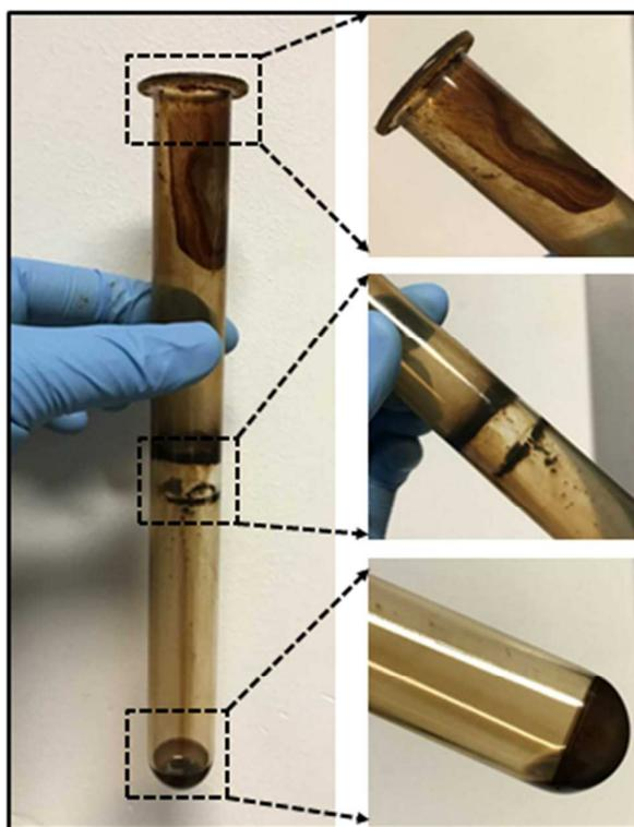
**Figure S6.** Samples left inside the VFD tube post VFD processing under continuous flow at 360 mJ, 7500 rpm with flow rate at 0.1 mL/min.
