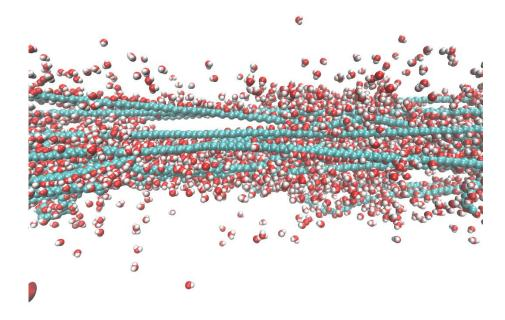
Snapshots of hydrogel with water content of 40 wt % when the strain is (a) 0, (b) 0.5, (c) 2.5 and (d) 4.5(the green, red, white represents PVA chain, oxygen of water, hydrogen of water respectively)
