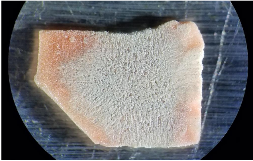
Figure S2. Image of a dried ossicle plate from the test of Strongylocentrotus fragilis sanded flat and mounted to a steel block prior to nanoindentation analysis.
