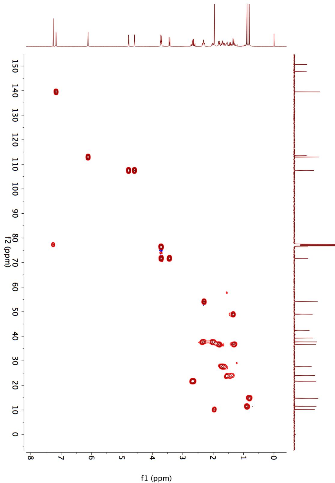
**Figure S53.** HMBC spectrum of compound **6** in  $\text{CDCl}_3$
