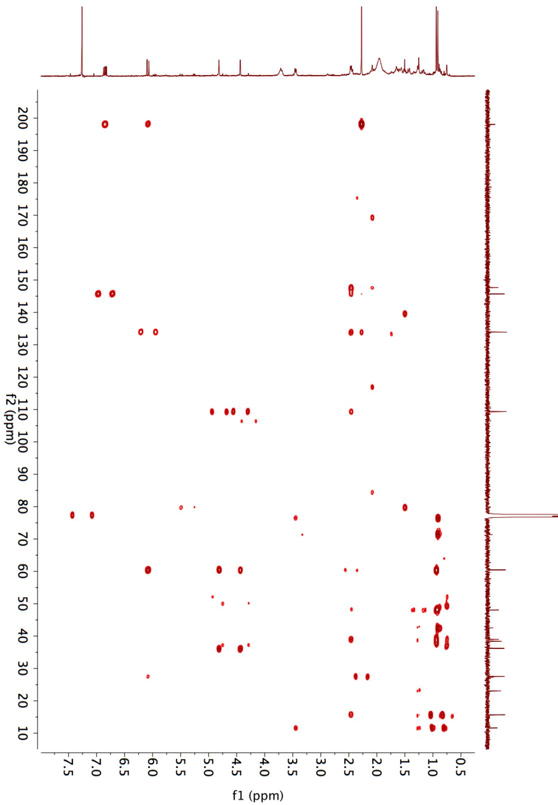
**Figure S44.**  $^1\text{H}$ - $^1\text{H}$  COSY spectrum of compound **5** in  $\text{CDCl}_3$
