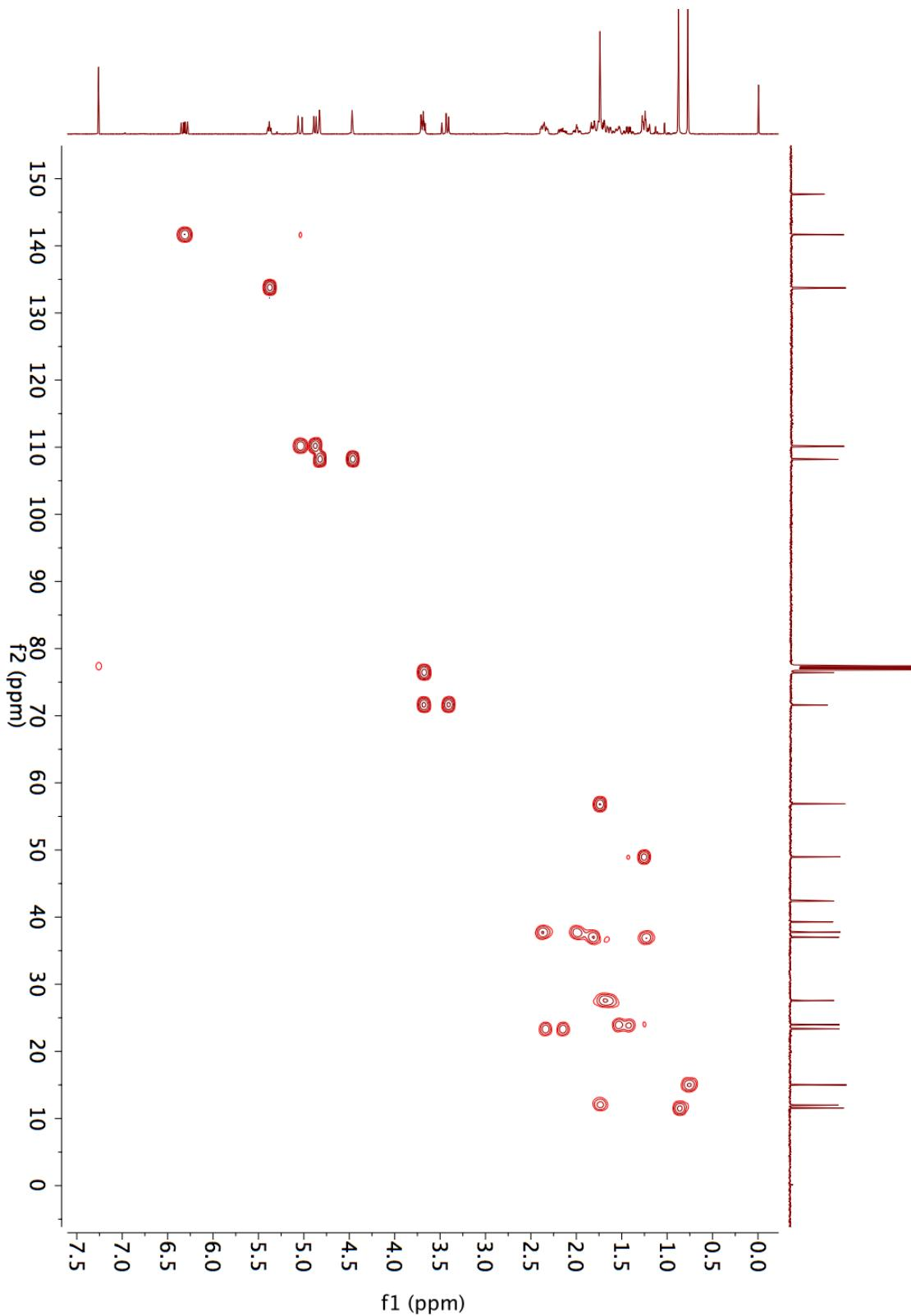
**Figure S62.** HMBC spectrum of compound 7 in  $\text{CDCl}_3$
