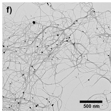
**Multi-Walled Carbon Nanotubes**
