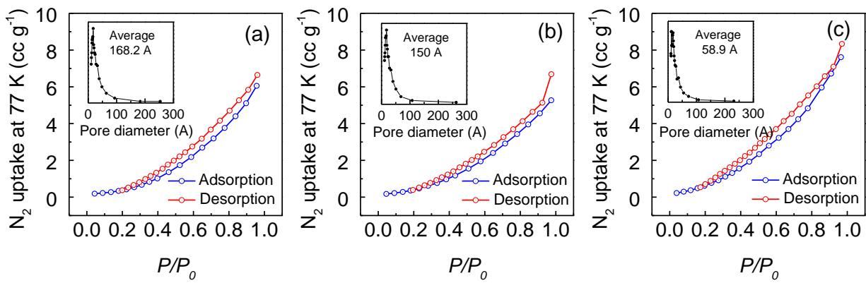
**Figure S3.** Nitrogen adsorption-desorption isotherms of (a) the pristine PVDF membrane, (b) PDA-coated PVDF membrane, and (c) TiO<sub>2</sub>-modified PVDF membrane. The insets show membrane pore size distributions.
