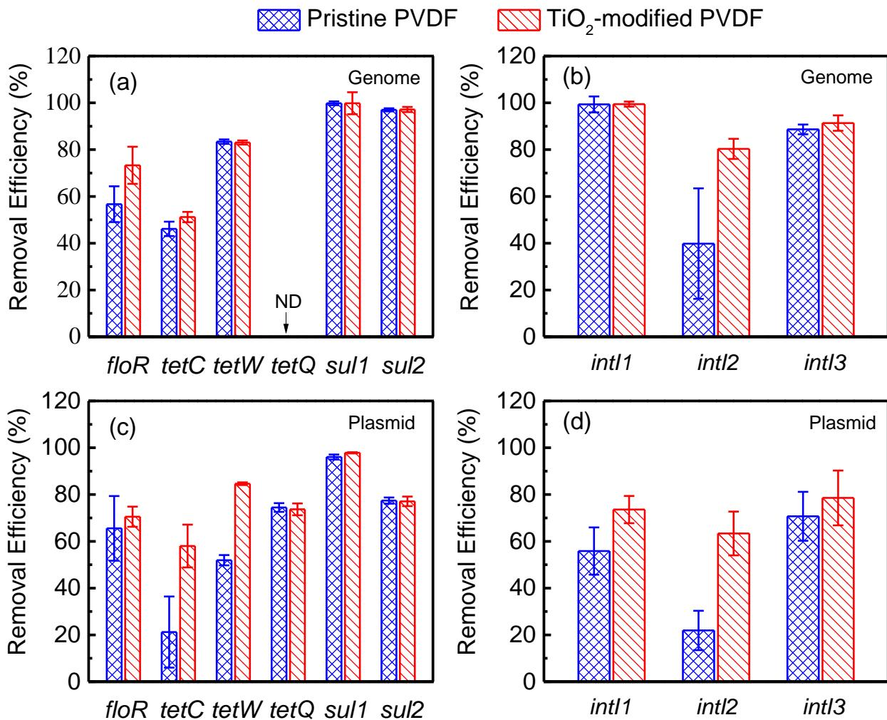
**Figure S5.** Removal efficiency of ARGs and integrons located in genome (a, b) and plasmid (c, d) by the pristine and TiO<sub>2</sub>-modified PVDF membranes evaluated in UF experiments.
