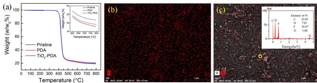
**Figure S2.** (a) Amount of  $\text{TiO}_2$  incorporated in PVDF membranes measured via TGA. (b) Areal distribution of  $\text{TiO}_2$  on the modified PVDF membrane surface analyzed by SEM-EDS. (c) Combined SEM and EDS elemental mapping images. The inset indicates EDS result from a single point scanning (indicated as yellow circle). TGA (SDT-Q600, TA Instruments Inc., USA) was carried out from 30 to 800 °C at a heating rate of 10 °C/min under nitrogen atmosphere.
