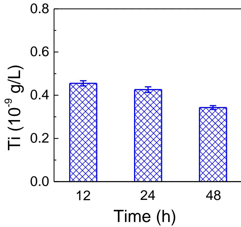
**Figure S7.** Amount of Ti leached to the permeate after UF experiments for 12, 24, and 48 h.
