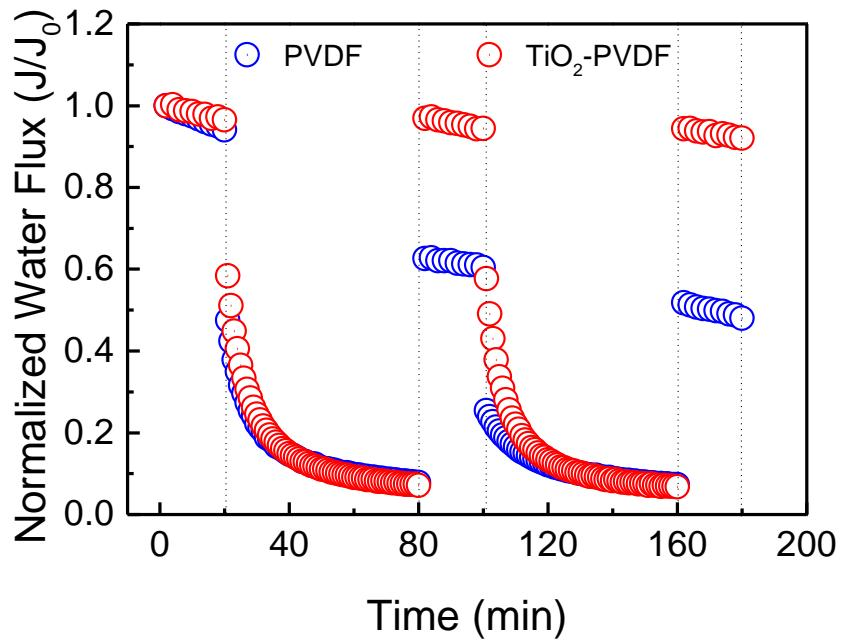
**Figure S6.** Normalized water flux for pristine PVDF membrane and  $\text{TiO}_2$ -modified PVDF membrane obtained from UF fouling experiments with wastewater effluent. Membranes were compacted for 3 h at 1.4 bar (20 psi) before UF experiments. Each fouling cycle comprised filtration of DI water for 20 min at applied pressure of 1.4 bar (20 psi) and secondary wastewater effluent for 60 min, followed by UV irradiation for 60 min.
