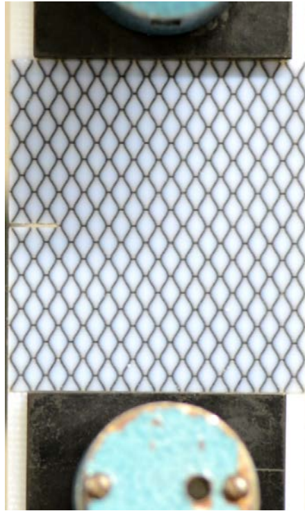
Figure 3.7 – Image of basic mechanical testing set up for Mode I single edge notched tensile testing. Grips are shown in black at the top and bottom of the image, moving up and down, respectively, to impart a tensile load on the hybrid samples
