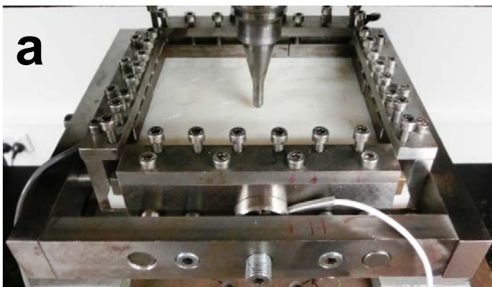
Figure 3.6 – a) Mechanical test set-up for osteomorphic assembly, with indenter and force sensors shown. Indenter moves down through the assembly to apply a concentrated point
