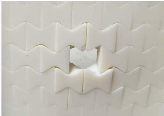
Figure 5.7 - a) Normalised load-displacement curves for assemblies of interlocked blocks with non-planar surfaces. The load and the displacement have been normalised in the same manner as in Figure 5.4. The solid lines correspond to the experimental curves and dashed lines to the computational curves. b) Damage to osteomorphic and square assemblies after mechanical testing
