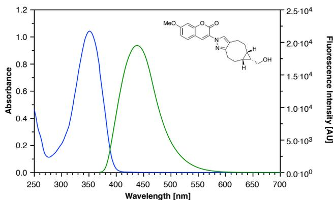
**Figure S6.** Absorption (blue trace (50  $\mu\text{M}$  in MeOH at 25  $^{\circ}\text{C}$ )) and fluorescence emission spectra (green trace) of pyrazole-coumarin **13**.
