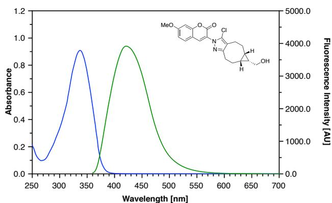
**Figure S7.** Absorption (blue trace (50  $\mu\text{M}$  in MeOH at 25  $^{\circ}\text{C}$ )) and fluorescence emission spectra (green trace) of chloropyrazole-coumarin **14**.
