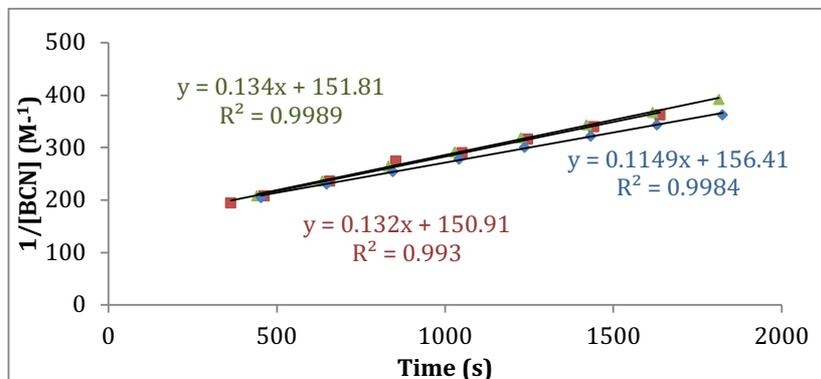
**Figure S1:** Kinetics measurement plots of BCN (**12**) and sydnone **4**. Decay of **4**: 3.95 (s, OCH<sub>3</sub>), 7.35 (s, CHsyd), 8.66 (s, CHar) and formation of the corresponding pyrazole **13**: 3.89 (s, OCH<sub>3</sub>), 8.13 (s, CHar), 8.16 (s, CHar).
