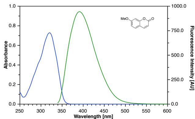
**Figure S3.** Absorption (blue trace (50  $\mu$ M in MeOH at 25  $^{\circ}$ C)) and fluorescence emission spectra (green trace) of 7-methoxycoumarin (**11**).
