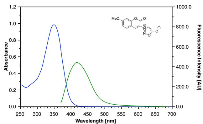
**Figure S4.** Absorption (blue trace (50  $\mu$ M in MeOH at 25  $^{\circ}$ C)) and fluorescence emission spectra (green trace) of sydnone-coumarin **4**.
