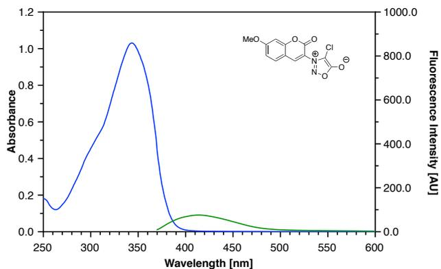
**Figure S5.** Absorption (blue trace (50  $\mu\text{M}$  in MeOH at 25  $^{\circ}\text{C}$ )) and fluorescence emission spectra (green trace) of chlorosydnone-coumarin **5**.
