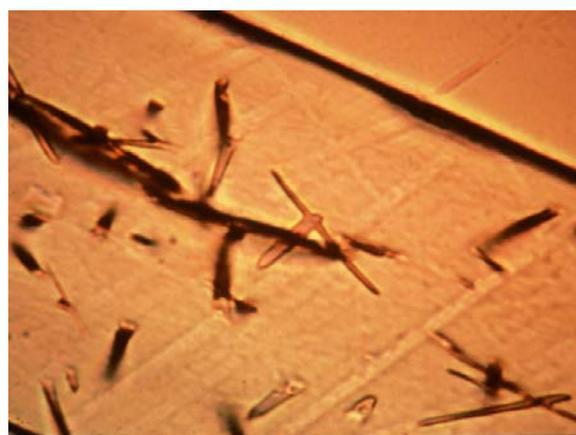
**Fig. C.2:** Confined fission track lengths in apatite. In order to determine the distribution of track lengths, measurements are made of the full length of horizontal tracks which are totally enclosed within the body of the crystal, which have been etched via fractures or other tracks which intersect the surface of the grain. Note that difference in width of the tracks is due to a difference in etch rate with crystallographic orientation, with a higher etch rate parallel to the C-axis
