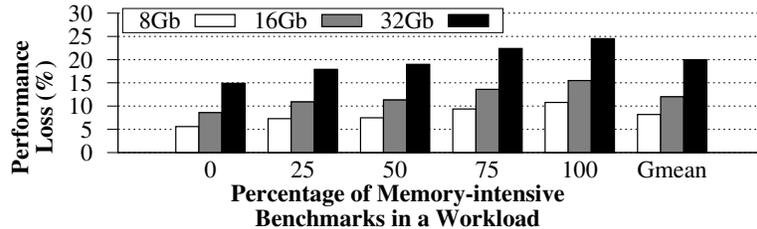
Figure 5.2. Performance degradation due to refresh.
