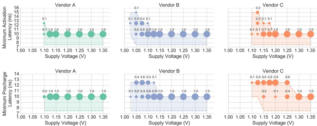
**Figure 7.5.** Distribution of minimum reliable latency values as the supply voltage is decreased for 31 DIMMs. The number above each point indicates the fraction of DIMMs that work reliably at the specified voltage and latency. Top row:  $tRCD_{min}$ ; Bottom row:  $tRP_{min}$ .
