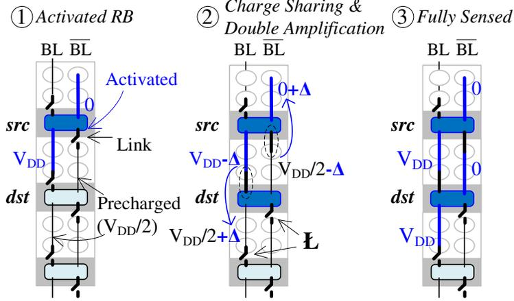
**Figure 4.4.** Row buffer movement process using LISA.
