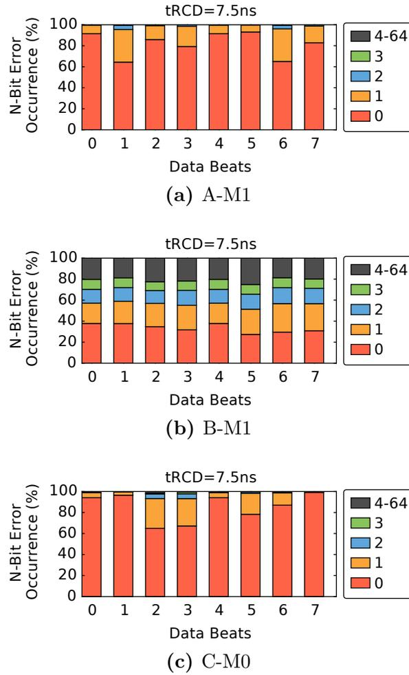
**Figure 6.8.** Breakdown of the number of error bits observed in each data beat of erroneous cache lines at  $t_{RCD}=7.5\text{ns}$ .
