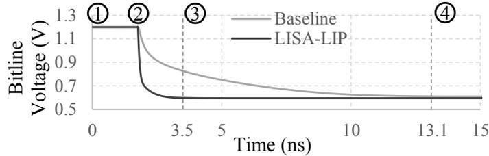
**Figure 4.11.** SPICE simulation of precharge operation.
