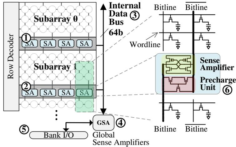
**Figure 2.5.** Bank and subarray organization in a DRAM chip.
