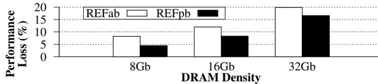
Figure 5.3. Performance loss due to  $REF_{ab}$  and  $REF_{pb}$ .
