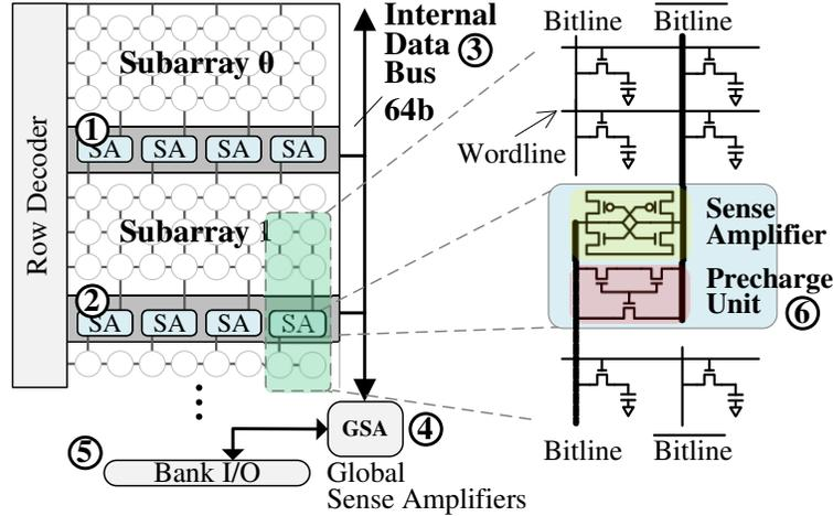
Figure 4.2. Bank and subarray organization in a DRAM chip.
