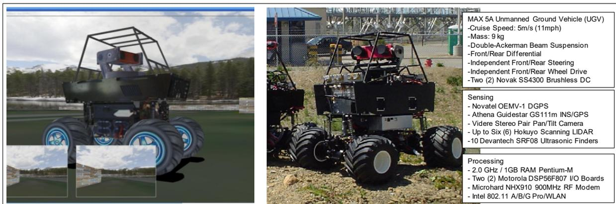
Figure 56. Senseta Corporation Max 5A UGV, Specifications (right) and Simulation Model (left)
