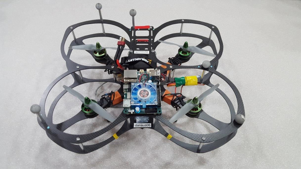
Figure A.4: The small quadrotor equipped with an ODROID-XU4 used for experimental validation of NPE (Ch. 3), EPC (Ch. 4), and Robust EPC (Ch. 5).
