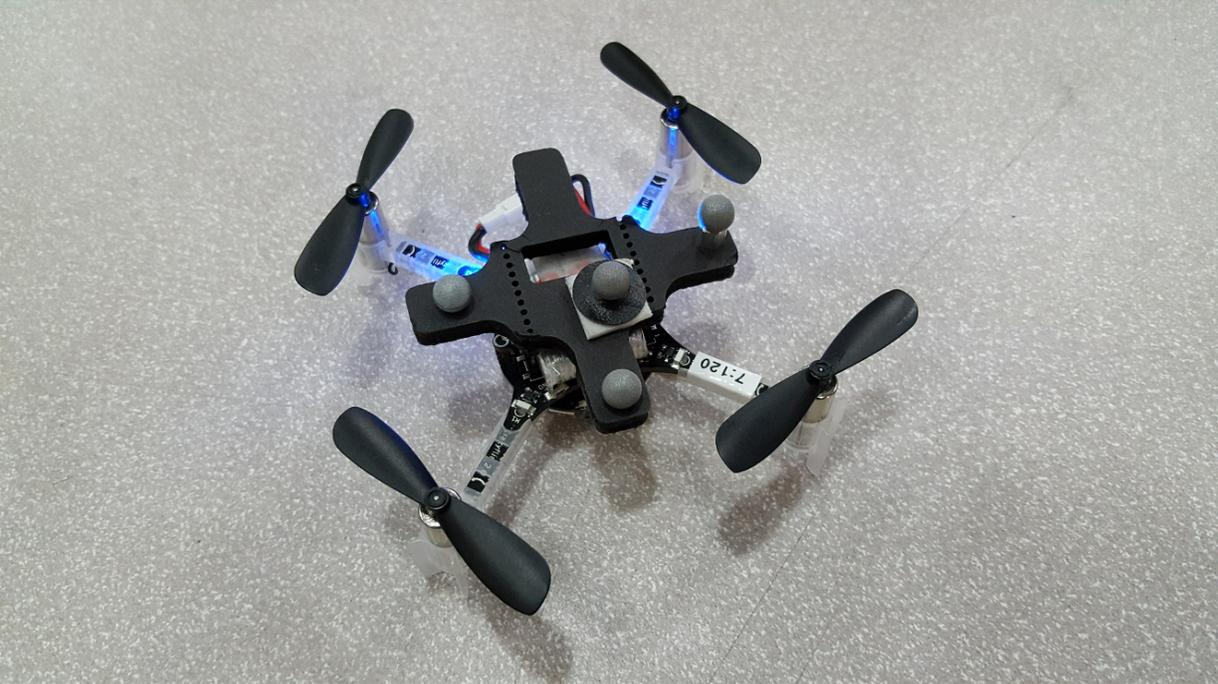
Figure A.5: The Crazyflie quadrotor used for experimental validation of the efficient explicit adaptive NMPC technique (Ch. 6).
