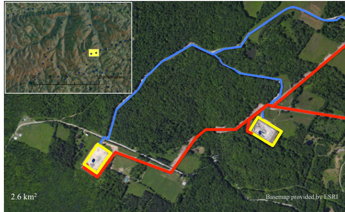
Figure 2: The three key components of Marcellus infrastructure include well pads (yellow), access roads (blue), and gathering lines (red)
