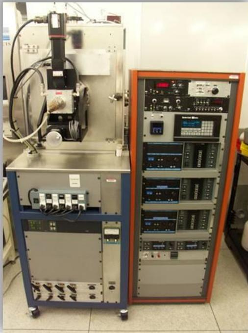
Figure 3-2 Custom 5-Target Sputtering System #2.
