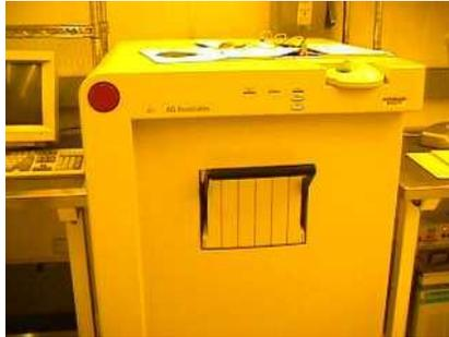
Figure 3-3 AG Associates Heat Pulse Rapid Thermal Annealing System.
