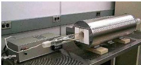
Figure 3-4 Tube Annealing Furnace.
