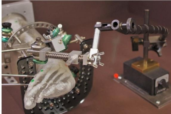
**Figure 6-20** Prismatic trajectory joint was positioned by the universal positioning arm and secured to the revolute trajectory joint.
