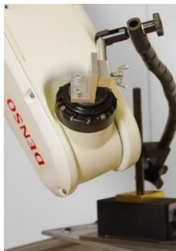
**Figure 6-17** Robot positioned the end effector in the calculated pose and the universal positioning arm was attached to the end effector via the adapter.
