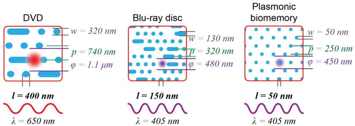
**Figure S13.** Comparison of various characteristics of a DVD, Blu-ray disc and plasmonic biomemory. (track pitch  $p$ , pit width  $w$ , minimum pit length  $l$ , laser spot size  $\phi$  and laser wavelength  $\lambda$ )
