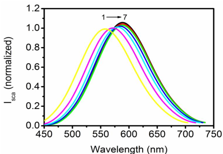
**Figure S5.** Representative scattering spectra of single Au@Ag NC-tsDNA<sub>17</sub> probe obtained at different times after adding 1 pM miR-21, showing that the  $\lambda_{\max}$  of the LSPR spectrum is redshifted, spectra 1-7: 0, 30, 60, 90, 120, 150, 180 min.
