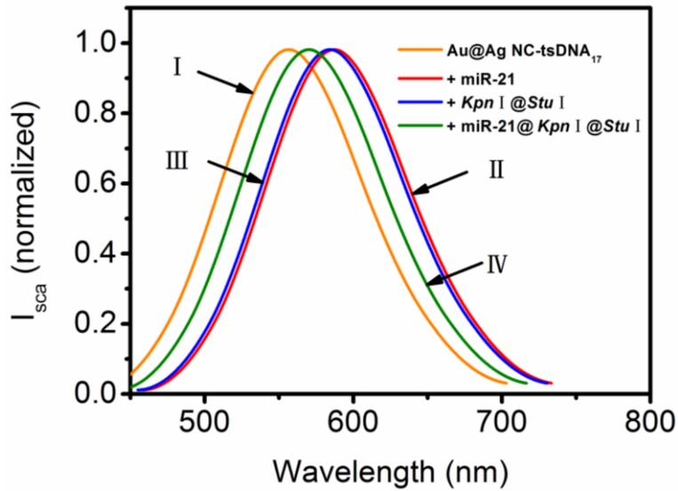
**Figure S12.** Typical scattering spectra of Au@Ag NC-tsDNA<sub>17</sub> probes before (I) and after addition of either miR-21 (II) or endonucleases (*Kpn*I and *Stu*I) (III) as well as both miR-21 and endonucleases (IV), showing the shift of  $\lambda_{\text{max}}$  of Au@Ag NC.
