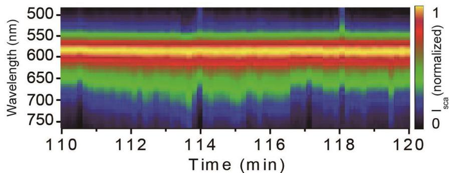
**Figure S7.** The scattering intensity ( $I_{sca}$ ) as a function of time when a single Au@Ag NC-tsDNA<sub>17</sub> probe hybridized with 1 pM of miR-21 during the interval from 110 to 120 min. The final concentration of tsDNA<sub>17</sub> and miR-21 in the used solutions is 1 pM.
