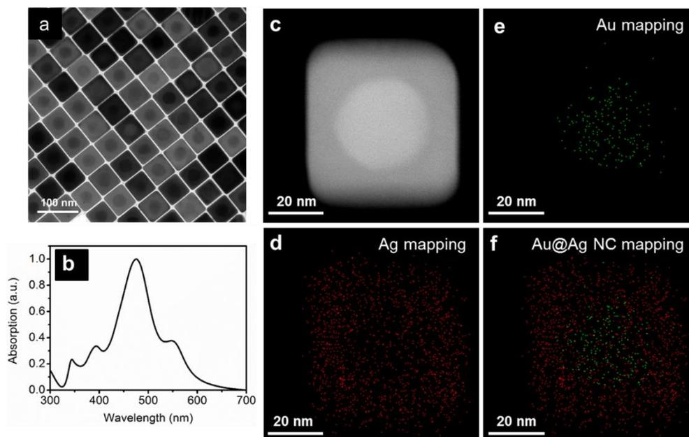
**Figure S1.** (a) TEM image of Au@Ag NCs with an average diameter of  $\sim 55$  nm. Scale bar, 100 nm. (b) Normalized UV-vis absorption spectrum for  $\sim 55$  nm Au@Ag NCs sample in aqueous solution. (c) Typical HAADF-STEM image of a Au@Ag NC. (d-f) Corresponding HAADF-STEM-EDS elemental mapping images of the Au@Ag NC in c. Scale bar, 20 nm.
