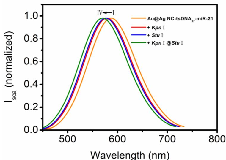
**Figure S10.** Typical scattering spectra of Au@Ag NC-tsDNA<sub>17</sub>-miR-21 nanoconjugates before (I) and after cleavage by endonucleases *Kpn*I (II), *Stu*I (III) and *Kpn*I@*Stu*I (IV), showing that the  $\lambda_{\text{max}}$  of nanoconjugate is blue shifted.
