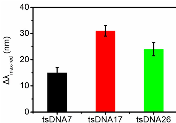
**Figure S6.** Peak shifts of three types of Au@Ag NC-tsDNA probes under the same reaction conditions. The  $\Delta\lambda_{\max\text{-red}}$  values were 15, 31, and 24 nm for tsDNA<sub>7</sub>, tsDNA<sub>17</sub>, and tsDNA<sub>26</sub>, respectively. The final concentration of tsDNA<sub>7</sub>, tsDNA<sub>17</sub>, tsDNA<sub>26</sub>, and miR-21 in all used solutions is 1 pM.
