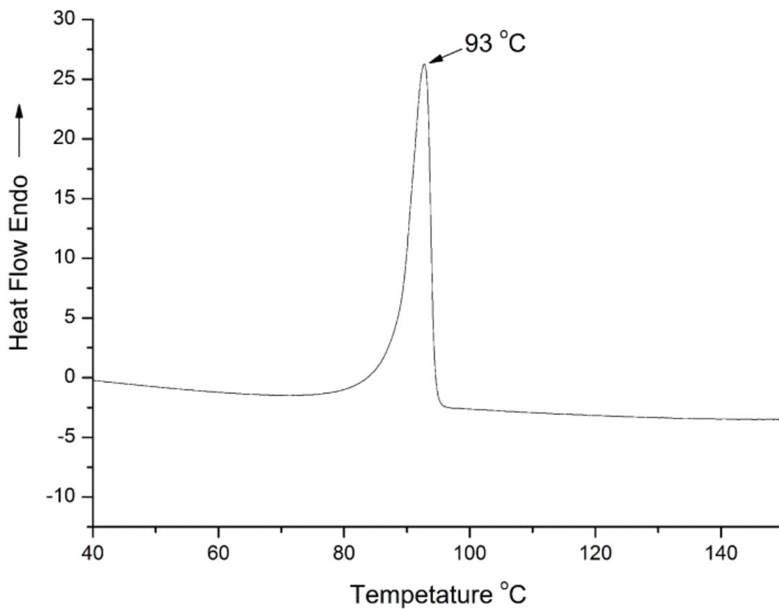
**Figure S6.** The melting point ( $T_m$ ) of  $M_{Se}$  measured by DSC.
