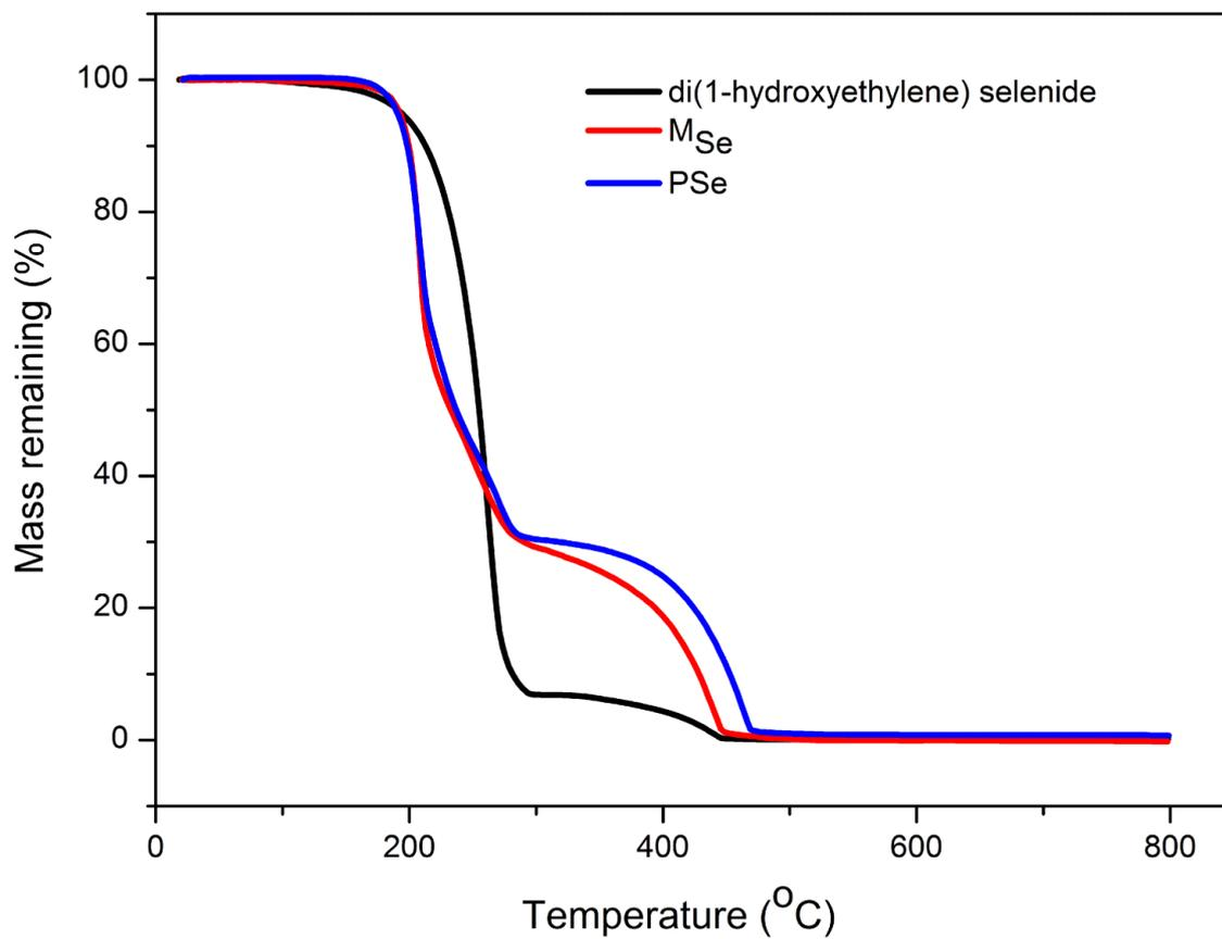
**Figure S8.** Thermo-gravimetric analysis of di(1-hydroxyethylene) selenide, M<sub>Se</sub> and PSe.
