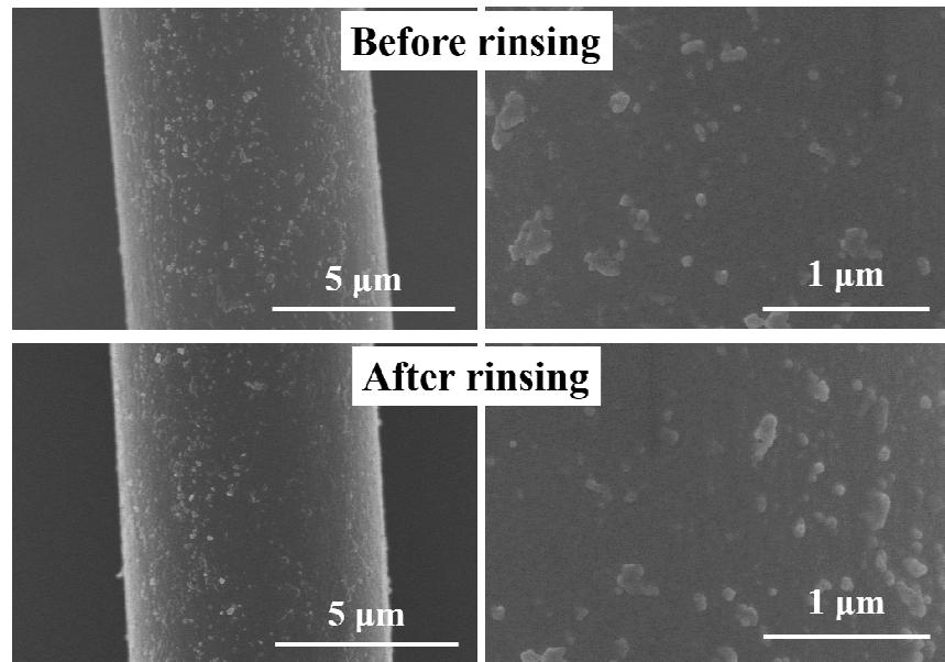
**Figure S2.** SEM images of the surfaces on CF-PDA/POSS before and after rinsing for about 3 h. As for rinsing test, CFs were fixed on the inner wall of a beaker by aluminum foil tape, then rinsing with water under high speed stirring (about 3000 r/min).
