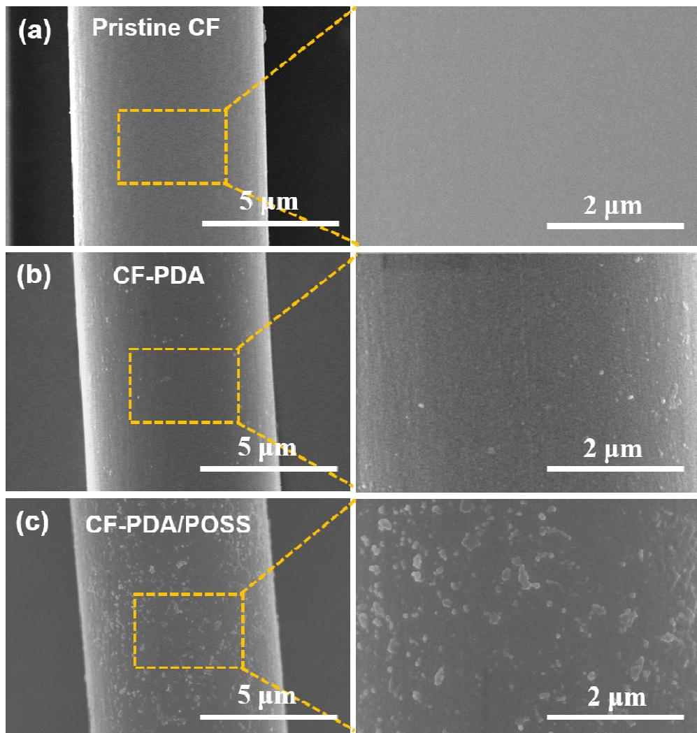
**Figure S3.** SEM images on the surfaces of CFs, including (a) pristine CFs, (b) CF-PDA, and (c) CF-PDA/POSS.
