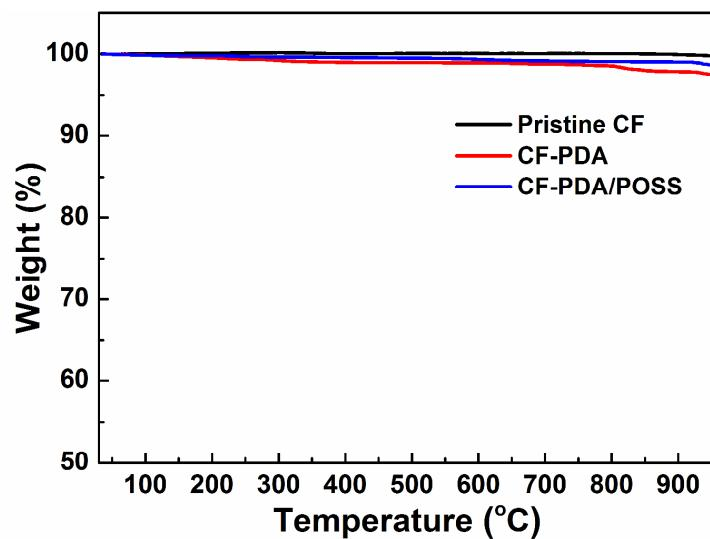
**Figure S4.** TGA traces of pristine CF (black line), CF-PDA (red line), and CF-PDA/POSS (blue line).
