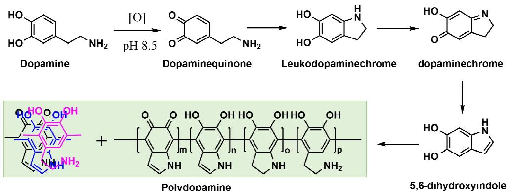
**Figure S1.** The typical polymerization mechanism of polydopamine (PDA).
