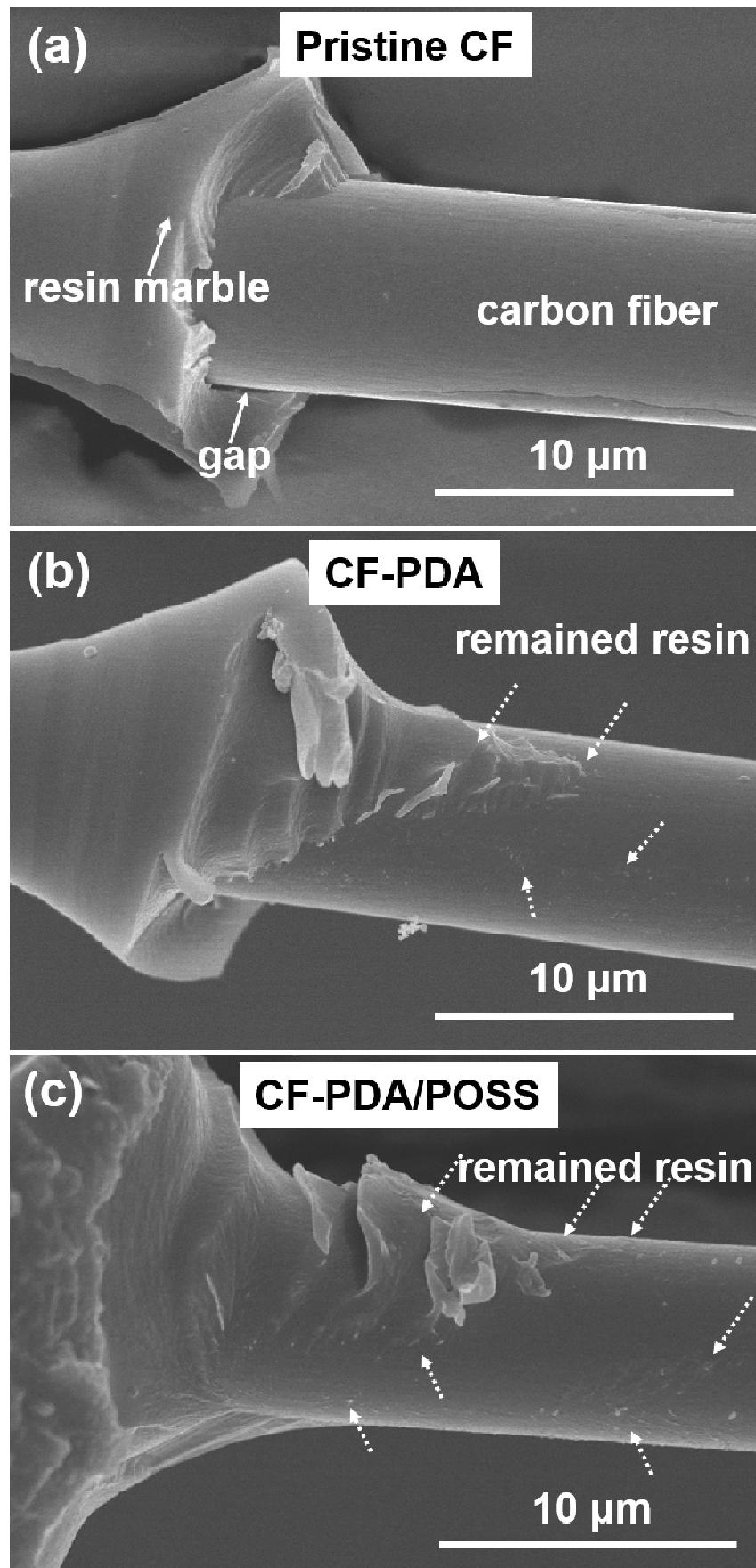
**Figure S5.** SEM images of the samples (a) the pristine CF, (b) CF-PDA, and (c) CF-PDA/POSS after IFSS measurement through pulling out the cured resin marbles from the single filament. The exposed fiber surface of pristine CF was almost neat and there appeared gap between fiber and resin. There remained few epoxy freagments on the surfaces of CF-PDA, more freagments on CF-PDA/POSS, simultanously showed benign connection between fiber and resin.
