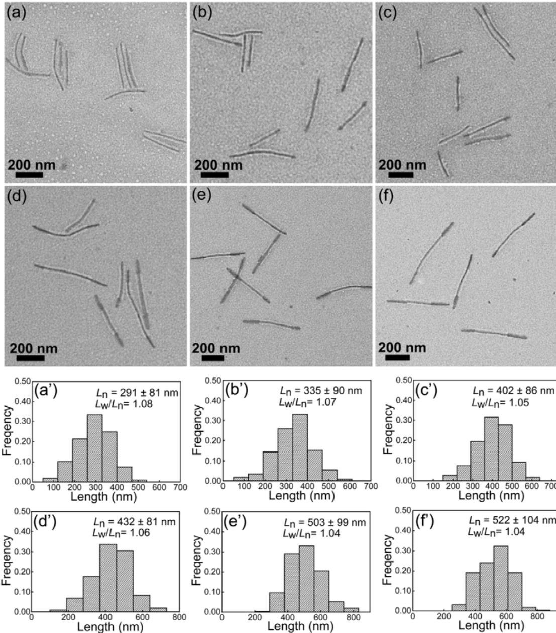
**Figure S12.** TEM images (a-f) and their corresponding histograms (a'-h') of the contour lengths of the micelles obtained by growing PFS<sub>35</sub>-*b*-P2VP<sub>400</sub><sup>Q</sup> unimer on PFS<sub>26</sub>-*b*-PNIPAM<sub>190</sub> seed micelles ( $L_n = 290 \pm 76$  nm,  $L_w/L_n = 1.07$ ). The aging times were (a) and (a') 10 min, (b) and (b') 100 min, (c) and (c') 1000 min, (d) and (d') 7 days, (e) and (e') 45 days, (f) and (f') 80 days, respectively.
