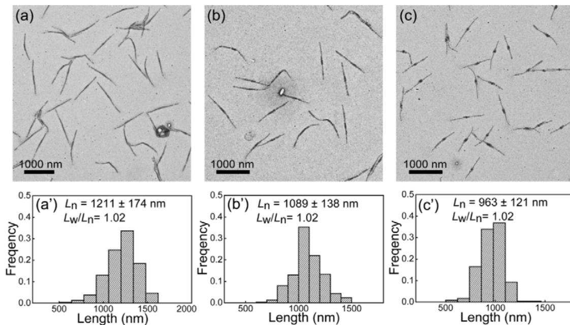
**Figure S3.** TEM images and the corresponding histograms of the contour length of the patchy micelles shown in Figure 1. The mass ratios of PFS<sub>35</sub>-*b*-P2VP<sub>400</sub> to PFS<sub>26</sub>-*b*-PNIPAM<sub>190</sub> are (a) and (a') 3:1, (b) and (b') 1:1, (c) and (c') 1:3, respectively. The unimer-mixture-to-seed weight ratio was 40:1.
