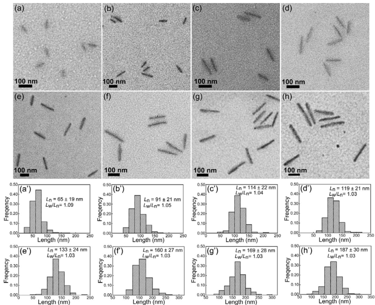
**Figure S10.** TEM images (a-h) and their corresponding histograms (a'-h') of the contour lengths of the micelles obtained by growing PFS<sub>35</sub>-*b*-P2VP<sub>400</sub><sup>Q</sup> unimer on PFS<sub>35</sub>-*b*-P2VP<sub>400</sub> seeds ( $L_n = 40 \pm 13$  nm,  $L_w/L_n = 1.11$ ). The aging times were (a) and (a') 10 min, (b) and (b') 100 min, (c) and (c') 1000 min, (d) and (d') 3000 min, (e) and (e') 7 days, (f) and (f') 30 days, (g) and (g') 60 days, (h) and (h') 110 days, respectively.
