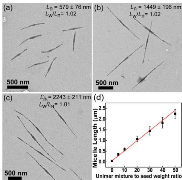
**Figure S14.** Controlling the length of the patchy cylindrical micelles by varying the weight ratio of unimer mixture (PFS<sub>26</sub>-b-PNIPAM<sub>190</sub>/PFS<sub>35</sub>-b-P2VP<sub>400</sub>, weight ratio 1:1) to seed. (a)-(c) are the TEM images of the patchy micelles in which the weight ratios of unimer mixture to seed are 10:1, 30:1, and 50:1, respectively. (d) shows that the length of the patchy micelles increased linearly as the weight ratio of unimer mixture to seed.
