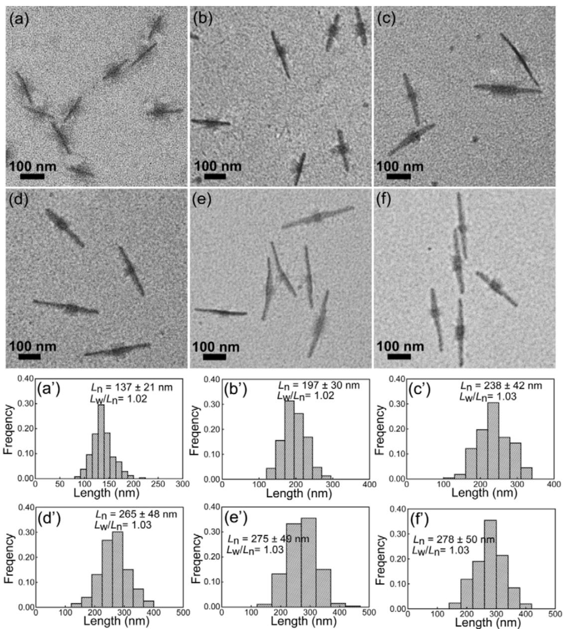
**Figure S5.** TEM images (a-f) and their corresponding histograms (a'-f') of the contour lengths of the micelles obtained by growing PFS<sub>26</sub>-*b*-PNIPAM<sub>190</sub> unimer on PFS<sub>35</sub>-*b*-P2VP<sub>400</sub> seeds ( $L_n = 40 \pm 13$  nm,  $L_w/L_n = 1.11$ ). The aging times were (a) and (a') 10 min, (b) and (b') 100 min, (c) and (c') 1000 min, (d) and (d') 7 days, (e) and (e') 60 days, (f) and (f') 110 days, respectively.
