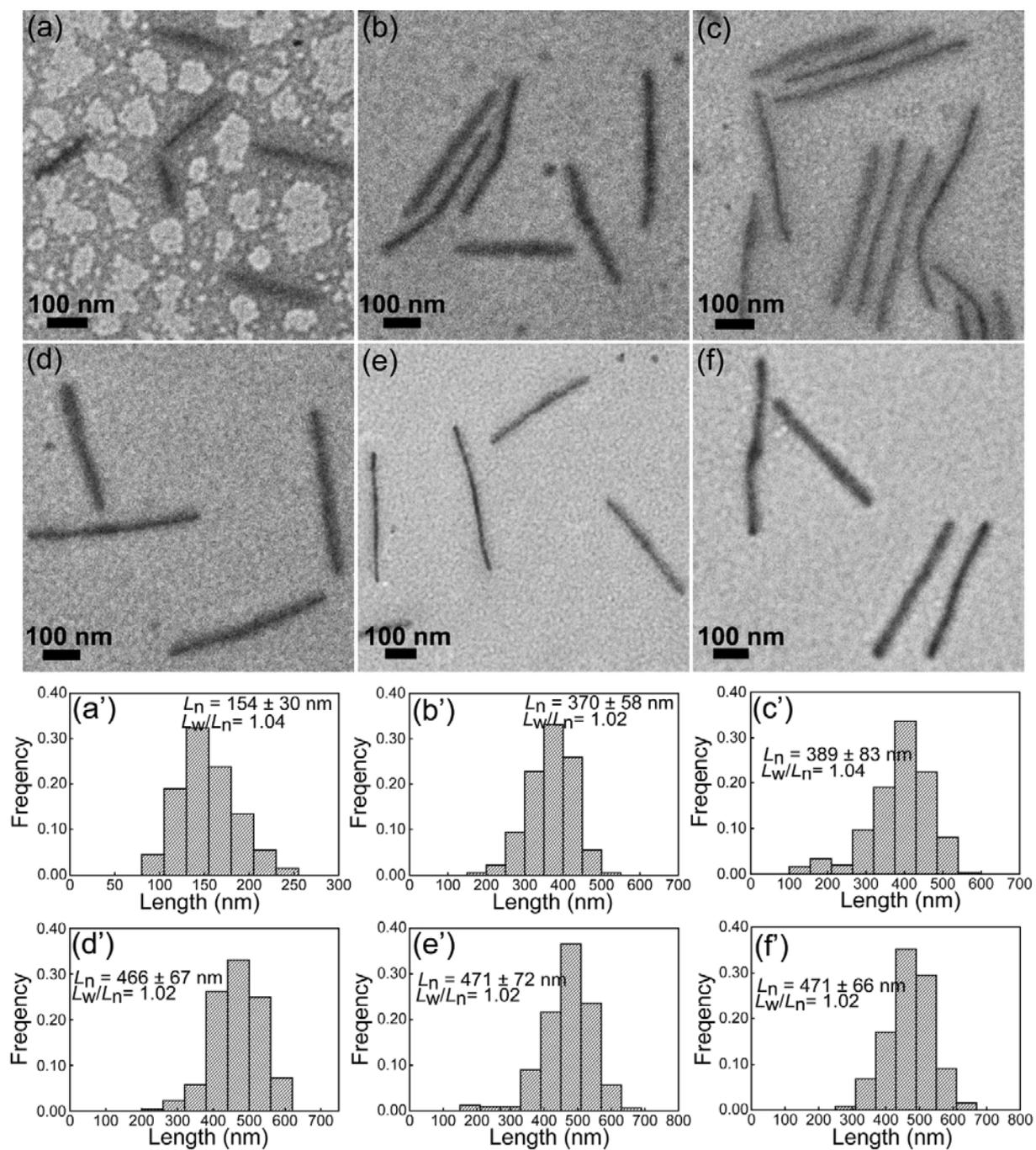
**Figure S6.** TEM images (a-f) and their corresponding histograms (a'-f') of the contour lengths of the micelles obtained by growing PFS<sub>35</sub>-*b*-P2VP<sub>400</sub> unimer on PFS<sub>35</sub>-*b*-P2VP<sub>400</sub> seeds ( $L_n = 40 \pm 13$  nm,  $L_w/L_n = 1.11$ ). The aging times were (a) and (a') 10 min, (b) and (b') 100 min, (c) and (c') 1000 min, (d) and (d') 7 days, (e) and (e') 60 days, (f) and (f') 110 days, respectively.
