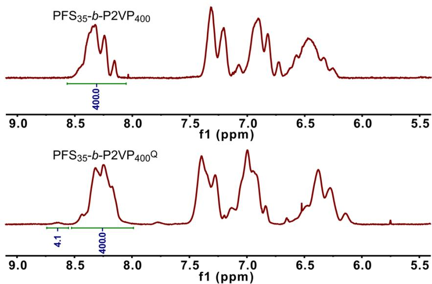
**Figure S9.**  $^1\text{H}$  NMR spectra of  $\text{PFS}_{35}\text{-}b\text{-P2VP}_{400}$  (upper spectrum) and  $\text{PFS}_{35}\text{-}b\text{-P2VP}_{400}^{\text{Q}}$  (bottom spectrum) in deuterated dimethyl sulfoxide. The degree of quaternization of the BCPs was evaluated to be 1 % ( $4.1/(400+4.1)$ ) by  $^1\text{H}$  NMR by comparing the integration of the  $\alpha$ -proton signal of the pyridinium units at 8.7 ppm to the  $\alpha$ -proton signal of the pyridine units at 8.3 ppm.
