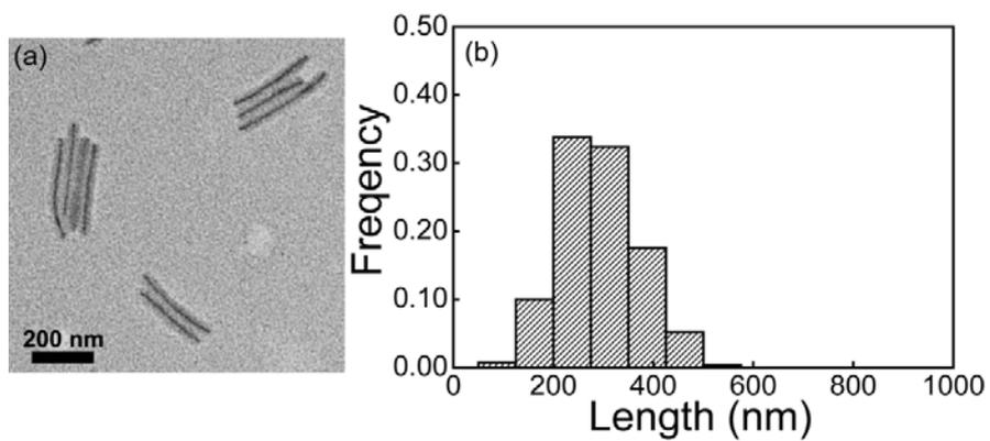
**Figure S11.** (a) PFS<sub>26</sub>-*b*-PNIPAM<sub>190</sub> seed micelles. (b) Histogram of the contour length of the seeds.  $L_n = 290 \pm 76$  nm,  $L_w/L_n = 1.07$ .
