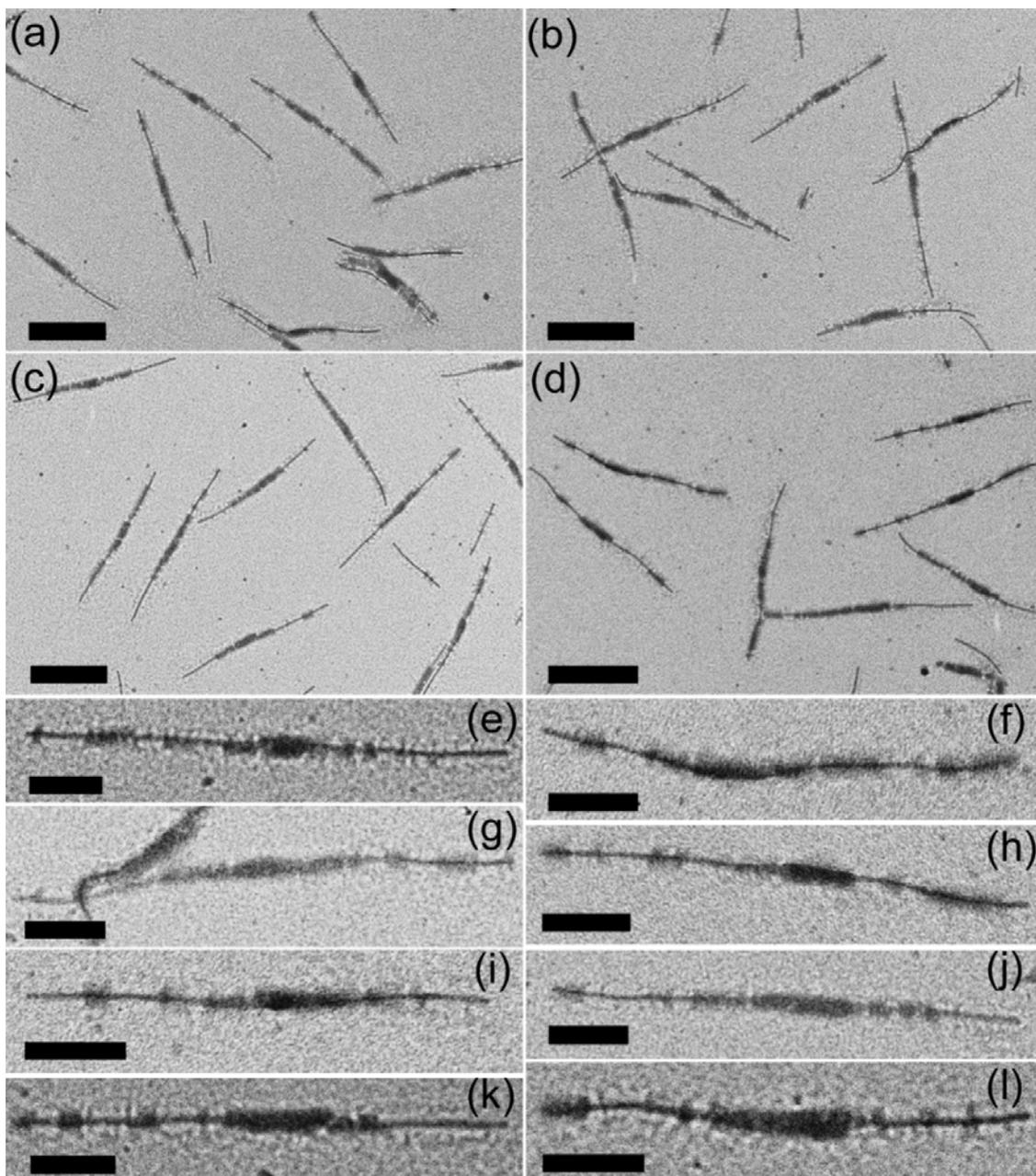
**Figure S2.** Additional TEM images of the patchy micelles shown in Figure 1a. The mass ratio of PFS<sub>35</sub>-*b*-P2VP<sub>400</sub> to PFS<sub>26</sub>-*b*-PNIPAM<sub>190</sub> is 1:1. The scale bars in (a)-(d) are 500 nm and in (e)-(l) are 200 nm.
