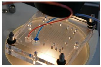
serpentine mixer, mounted using silicon ferrules.
