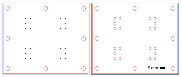
**Figure B2A**: Design of PMMA chipholder bottom plate, with engraved spots for alignment of the fluidic connections. The holder is produced from cast PMMA of 6 mm thickness using the Trotec Speedy 300 laser cutter. Cutting is done at 500 dpi, 10,000 Hz, power 100, speed 0.3. Engraving of dots: 500 dpi, 10,000 Hz, power 100, speed 3.
