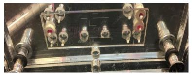
**Figure B3: Detail of the PMMA holder holding the FFDG droplet generator.** For this experiment, Perlast ferrules and an adapter plate (2 mm thickness, with 3.4 mm holes to fit the SS ferrule rings placed directly below the top plate) were used.
