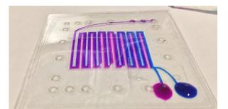
Figure B7: Example of large 50 x 50 mm foil chip design (laser-cut serpentine mixer, 300 µm channel width) filled with dyed water. The additional holes are in the (universal) top layer allow modification of the channel pattern using scissor or knife before assembly.
