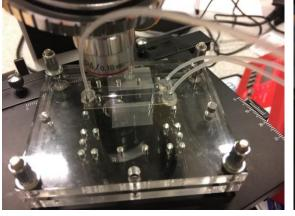
**Figure B5: Assembled chip PMMA holder** holding an 15 x 45 mm Y reactor foil chip (the channel of which was enlarged to 0.3 mm by scissors before assembly) and connected to the tubing using silicon ferrules. With this experiment a Calcite precipitate is formed from 0.025 M CaCl2 and 0.1 M NaHCO3 (for details see figure 7 of the main article). The reaction is observed using the 40x magnification of a standard microscope.
