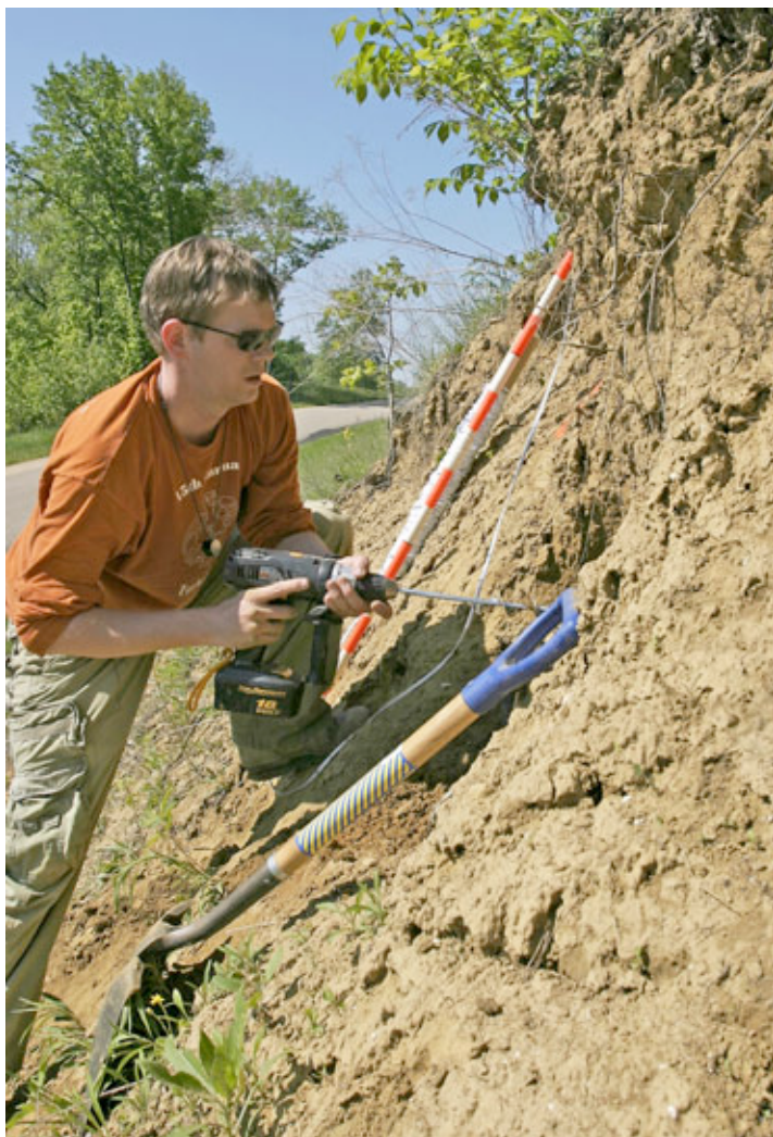
Figure 3.3A. Auger sampling at Big Platte.
