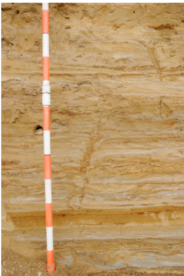
Figure 2.7B. Closeup view of laminated silt at Kulas-1 showing root traces and deformed bedding (near base). Color bands on Jacobs Staff are 10 cm.
