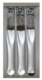
Figure 9 Water flotation tests showing the effectiveness of surfactants in altering the wettability of crude oil-aged BF rock exposed to surfactant solutions for 24 h (left: No surfactant; center: STEOL CS-330; right: surfactin).
