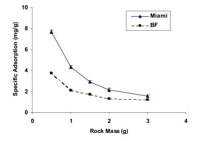
Figure 1 Adsorption of 1.44 mmol/l STEOL CS-330 vs. mass of crushed BF and Miami rocks. Error bars = 1 Std. Dev., n = 3
