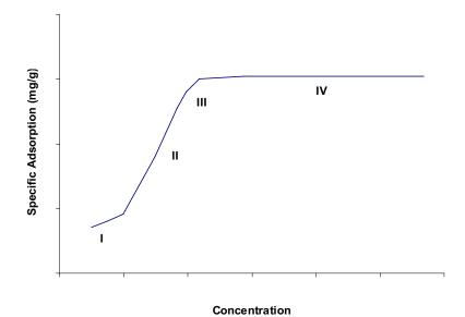
Figure 6 Typical adsorption isotherm of surfactant on rock indicating four regions (after Tabatabai *et al.* 1993)
