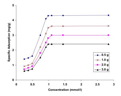
Figure 3 STEOL adsorption isotherms on different masses of crushed BF rock to show decline in adsorption with increasing rock mass
