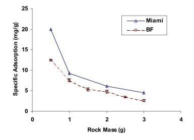
Figure 2 Adsorption of 0.37 mmol/l surfactin vs. mass of crushed BF and Miami rocks. Error bars = 1 Std. Dev., n = 3
