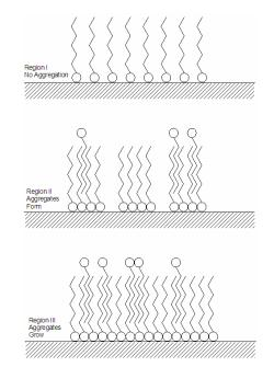
Figure 7 Suggested physical bases for the first three regions seen in a typical adsorption isotherm (after Sharma 1995)
