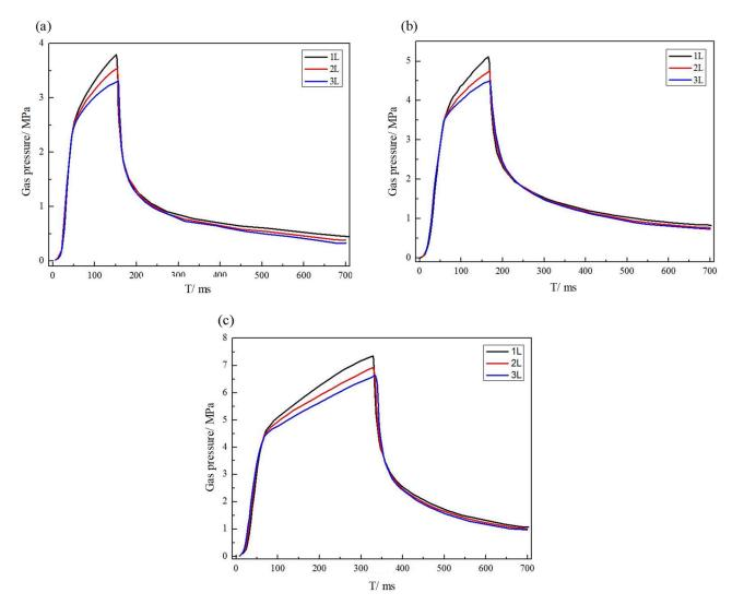
FIGURE 7: p-t curve of high pressure nitrogen fracturing under different design gas volume conditions. (a) V=1L; (b) V=2L; (c) V=3L.
