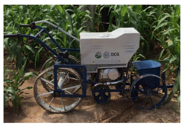
Supplemental Figure 2. Motorized planter/weeder developed in Mali
