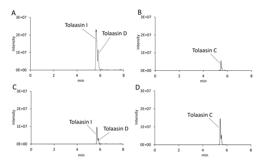
LC-MS chromatograms in selected ion recording (SIR) mode at m/z 994 [M+2H]<sup>2+</sup> for tolaasin I and D (panels A and C), and at m/z 1003 [M+2H]<sup>2+</sup> for tolaasin C (panels B and D). Panels A and B, the extract of tolaasins treated in PBS ; panels C and D, the extract of tolaasins treated with K3-5.
