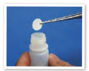
Insertion of exposed pad into Small Shipping Vial.
