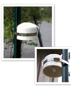
Ogawa Passive Sampler installed in Ozone Shelter.
