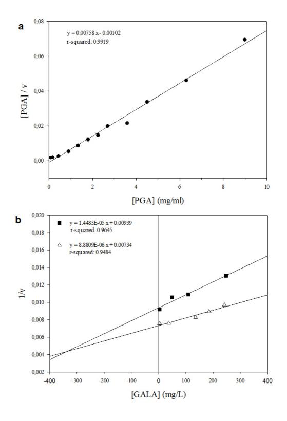
Fig. S4. (a) Hanes-Hultin plot used to determine the  $V_{MAX}$  and  $K_M$  values for PGA. (b) Dixon plot used to calculate the inhibition constant,  $K_i$ , for the enzymatic end-products of PGA hydrolysis. Two different substrate concentrations were employed in this assay: ( $\blacksquare$ ) 0.375 and ( $\Delta$ ) 0.4375 mg/ml; for each one, PG activity was measured in the presence of increasing amounts of end-products, expressed as [GALA].
