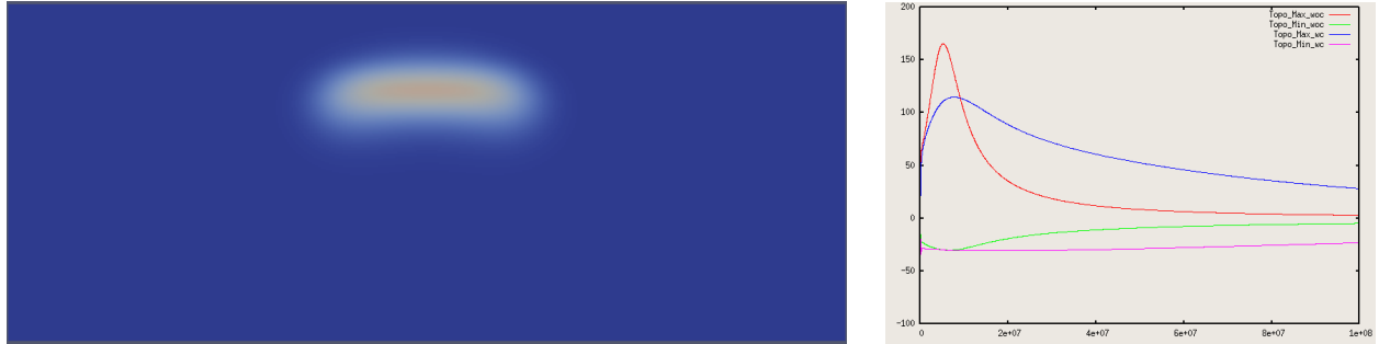
Figure 25: Adding a viscous crust to a model with surface topography. The thermal anomaly spreads horizontally as it collides with the highly viscous crust (left). The addition of a crustal layer both dampens and delays the appearance of the topographic maximum and minimum (right).
