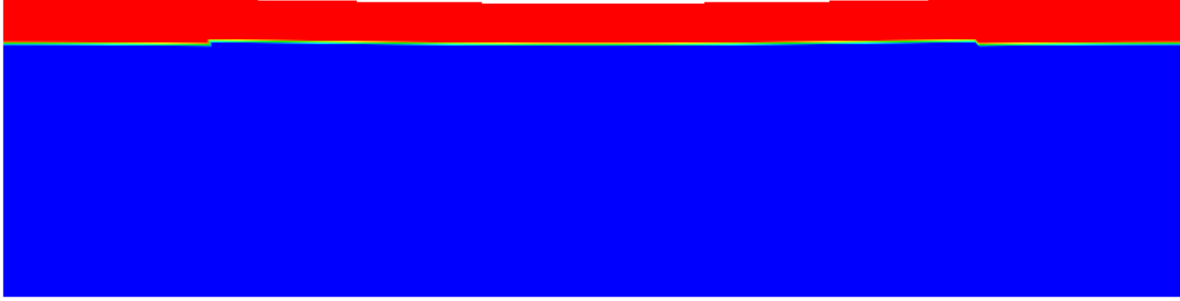
Figure 76: Setup for the topography relaxation benchmark. The box is 2800 km wide and 700 km high, with a 100 km lid on top. The lid has a viscosity of 10^{23} Pa s, while the mantle has a viscosity of 10^{21} Pa s. The sides are free slip, the bottom is no slip, and the top is a free surface. Both the lid and the mantle have a density of 3300 \text{ kg/m}^3 , and gravity is 10 \text{ m/s}^2 . There is a 7 km sinusoidal initial topography on the free surface.
