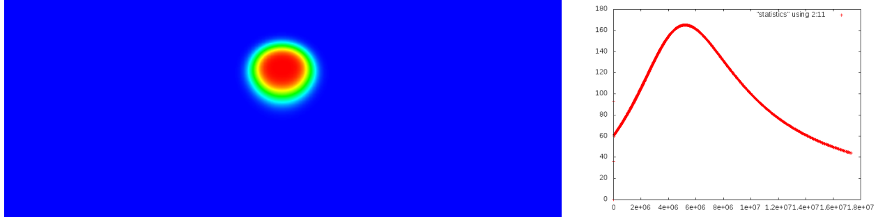
Figure 24: Evolution of surface topography due to a rising blob. On the left is a snapshot of the model setup. The right shows the value of the highest topography in the domain over 18 Myr of model time. The topography peaks at 165 meters after 5.2 Myr. This cookbook may be run with the cookbooks/free-surface.prm input file.
