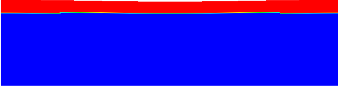
Figure 89: Setup for the topography relaxation benchmark. The box is 2800 km wide and 700 km high, with a 100 km lid on top. The lid has a viscosity of 10^{23} Pa s, while the mantle has a viscosity of 10^{21} Pa s. The sides are free slip, the bottom is no slip, and the top is a free surface. Both the lid and the mantle have a density of 3300 \text{ kg/m}^3 , and gravity is 10 \text{ m/s}^2 . There is a 7 km sinusoidal initial topography on the free surface.
