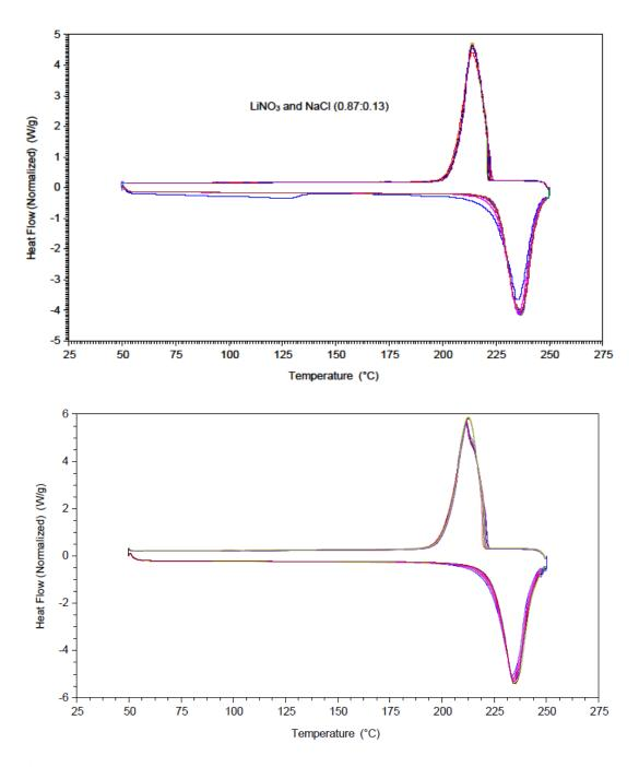
**Figure 1** The measured temperature heat flow graphs for the charging and discharging processes with the DSC (a) heating/cooling rate of 10 °C/min; (b) heating/cooling rate of 15 °C/min.
