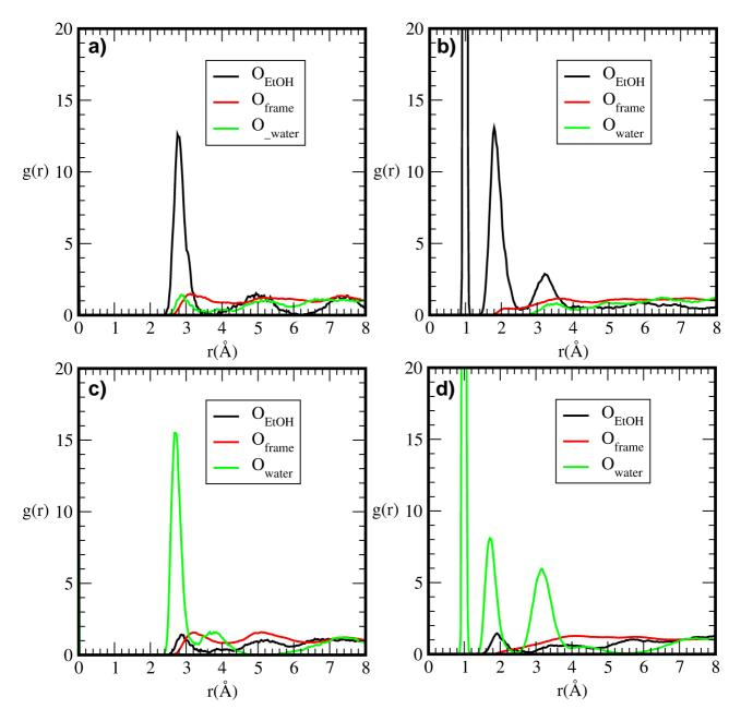
**Figure S4.** Pair distribution functions g(r) obtained from the room-temperature FPMD simulation of Si-FER-4EtOH-8H<sub>2</sub>O relative to  $P=P_{amb}$  (rev) (release to room pressure conditions). The reported g(r)'s are relative to: EtOH oxygen atoms, panel a; EtOH hydroxyl protons, panel b; water oxygen atoms, panel c; water protons, panel d.
