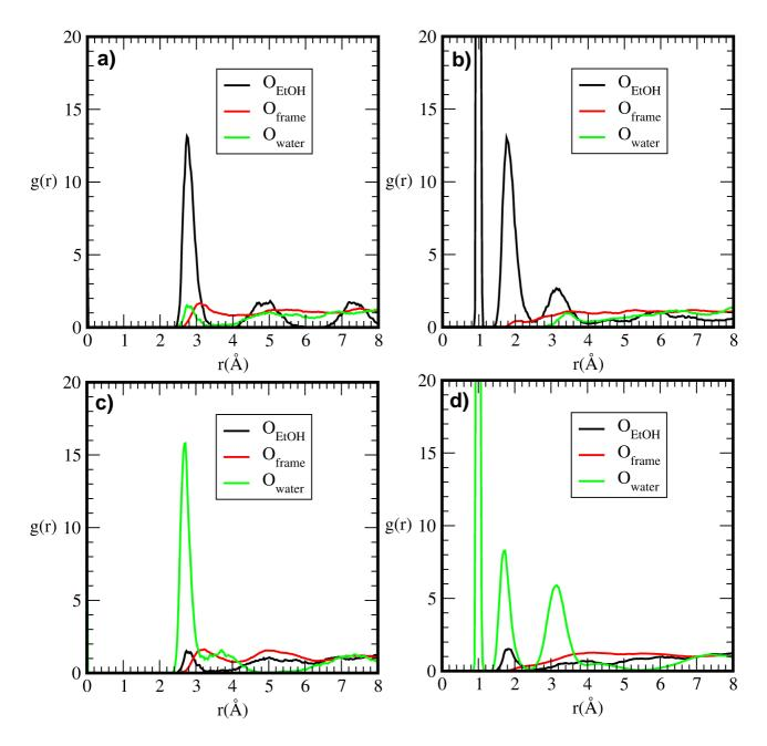
**Figure S3.** Pair distribution functions g(r) obtained from the room-temperature FPMD simulation of Si-FER-4EtOH-8H<sub>2</sub>O relative to *P*=0.84 GPa. The reported g(r)'s are relative to: EtOH oxygen atoms, panel a; EtOH hydroxyl protons, panel b; water oxygen atoms, panel c; water protons, panel d.
