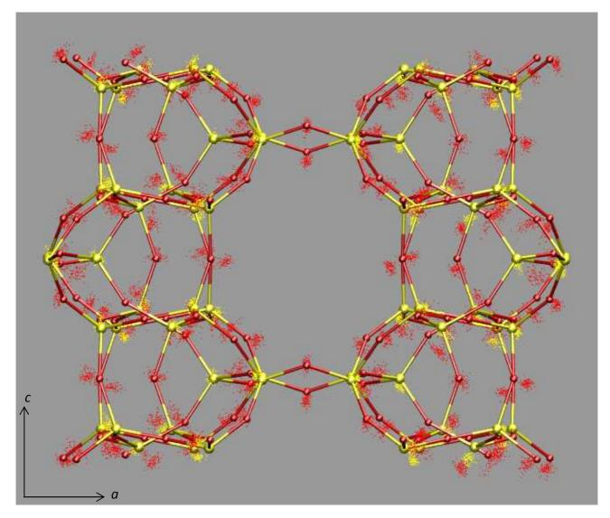
**Figure S2.** Comparison between the positions of the Si-FER framework atoms obtained from the refinement of the X-ray data collected at 0.84 GPa (ball-and-stick representation) and the corresponding atomic positions sampled at 10 fs intervals along the FPMD simulation (dots representation). Atom color codes: Si=yellow; O=red.
