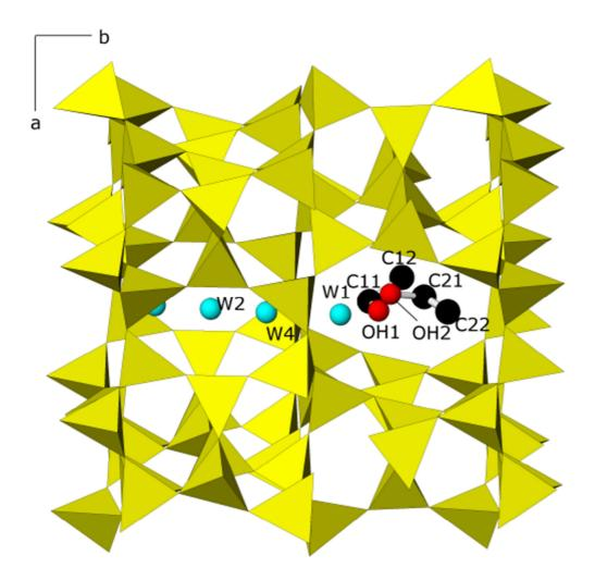
**Figure S1.** Graphical representation of the structure obtained from the refinement of the powder data collected for Si-FER compressed in e.w. (1:3) at 0.84 GPa. Atom labels as in Table S2. Atom colors: Si tetrahedra: yellow; O (water): cyan; EtOH oxygen positions (OH1, OH2): red, EtOH carbon position (C11, C12, C21, C22):black.
