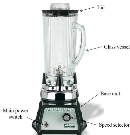
Figure 5.1: The mixing device used in the second phase of the experimental work.
