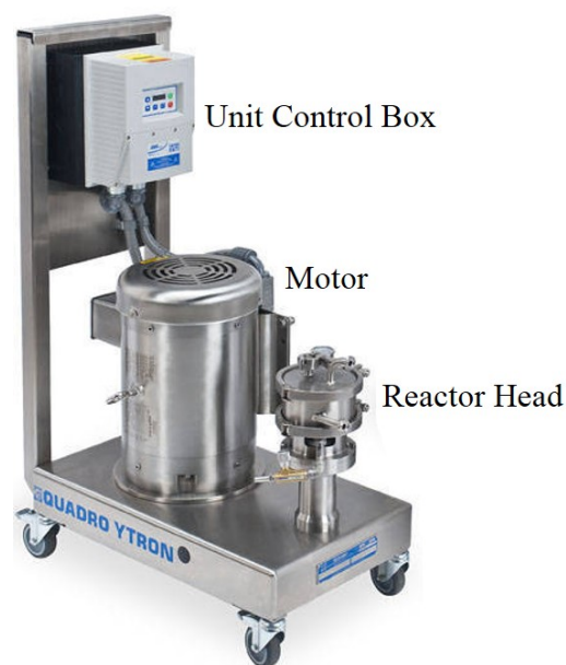
Figure 5.8: The device used to produce the micronised emulsion binder.
