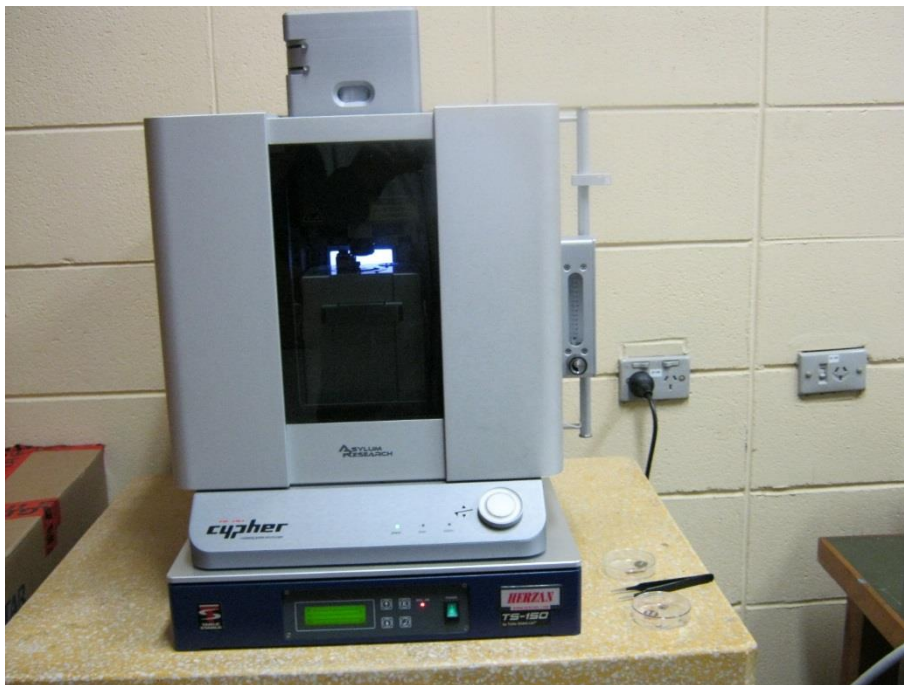
Figure 2.14: AFM from Asylum Research (Cypher scanning microscope) used in this project.
