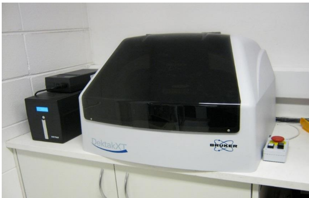
Figure 2.11: DektakXT stylus profiler used to measure the thickness of films.
